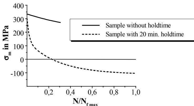
**Figure 4:** Example of mean stress development at 700 °C
