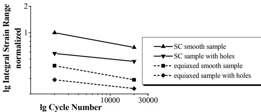
**Figure 7:** Comparison with a conventional cast superalloy
