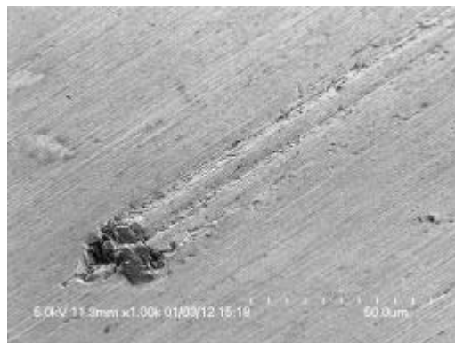
Fig.7 SEM micrograph of the corrosion pit
