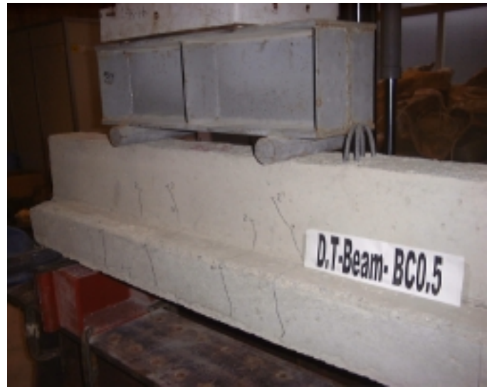
Photo 2: Mode of failure of polypropylene fibers beam
