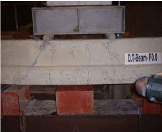
Photo 1: Mode of failure of control beam
