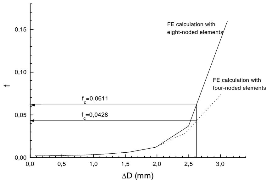
Figure 3: Determination of critical void volume fraction
