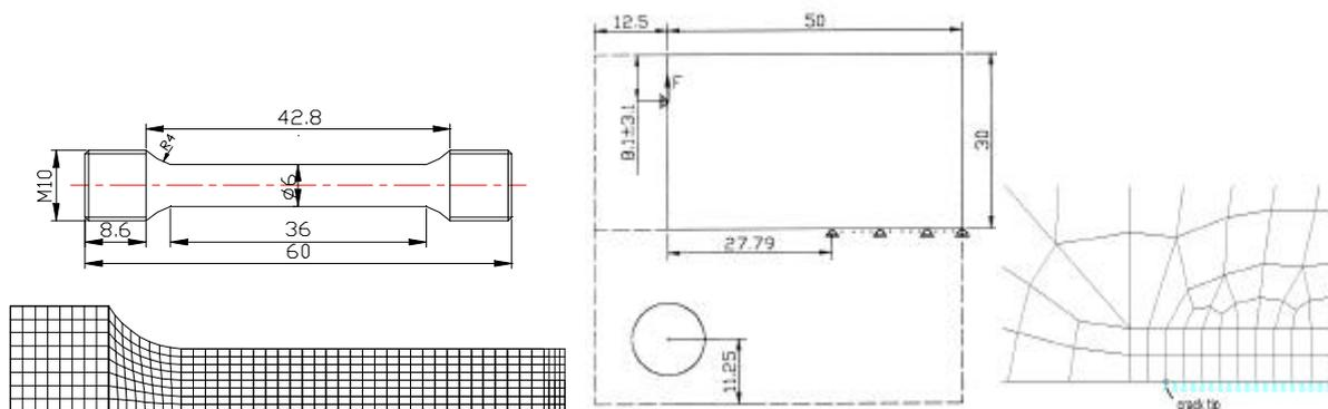
Figure 1: Tested specimens - dimensions and FE meshes
