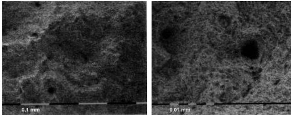
Figure 5: SEM micrographs of crack initiation in the center of smooth specimen
