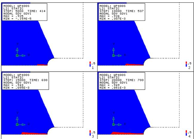
**Figure 3(c):** Distributions of damage,  $\omega$ , for different times: plane stress case,  $\alpha = 0.15$
