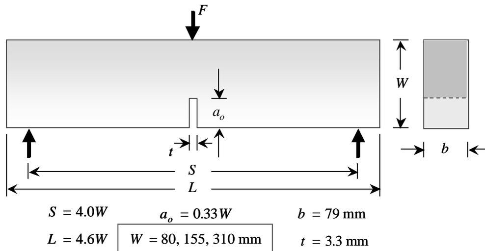
**Figure 1.** Single edge specimen loaded in bending, SE(B)
