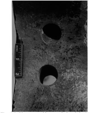
**Figure 4:** Ligament cracking at a tube bore hole viewed from the ID of a header.
