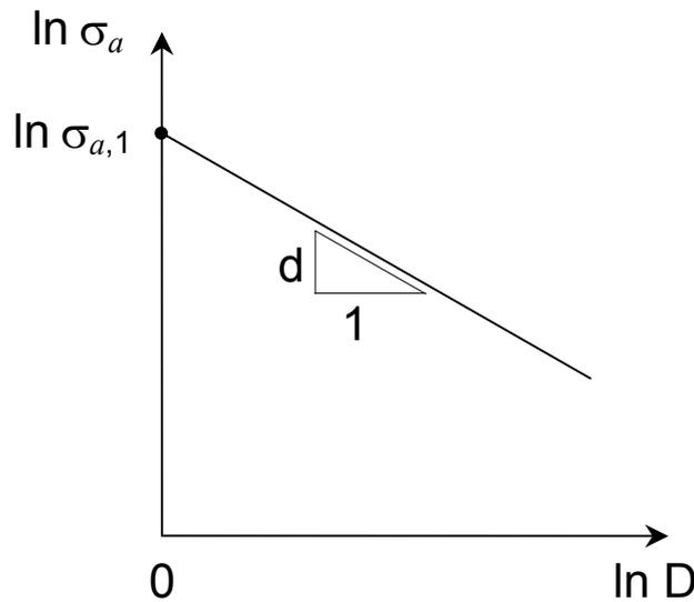
Figure 2: Monofractal scaling law for fatigue strength  $\sigma_a$
