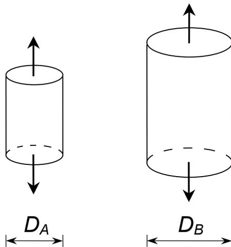
Figure 1: Geometrically similar cylinders under cyclic axial loading
