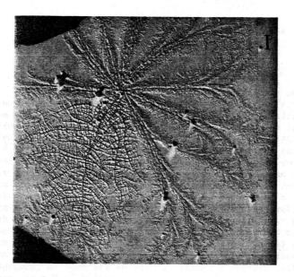
18. Electron micrograph of an incipient spherulite of polypropylene prepared by crystallization of a polymer fraction  $(M_{\rm W}=70\times10^3)$  in a 0.004% solution in A-chloronapthalene and subsequent rapid cooling (indicating
