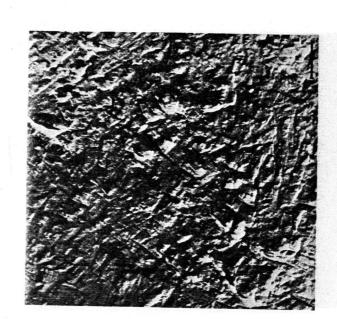
g.13. Electron micrograph of replica of portion of fracture surface of an annealed bulk sample of polypropylen molded at 16,900 psi (indicating mar corresponds to 0.5 μ).
