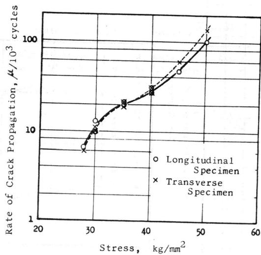
Fig. 5 Rate of crack propagation vs. stress levels.
