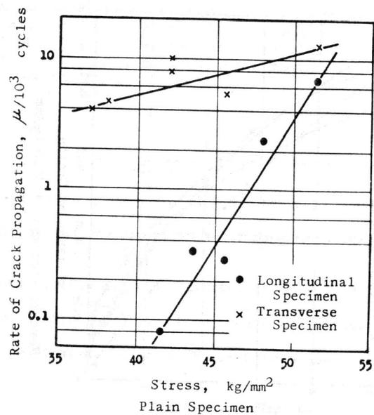
Fig. 4 Rate of crack propagation vs. stress levels.
