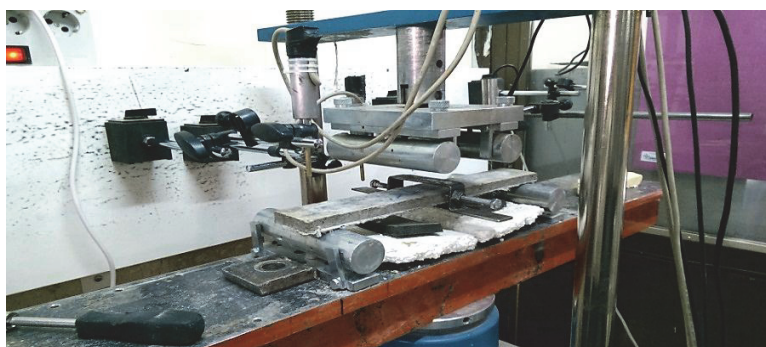
Figure 2: Four-point bending machine.
