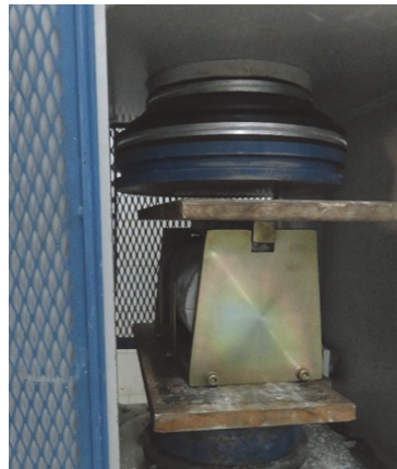
Figure 1: Cylindrical sample under sample splitting tensile test (Brazilian test).
