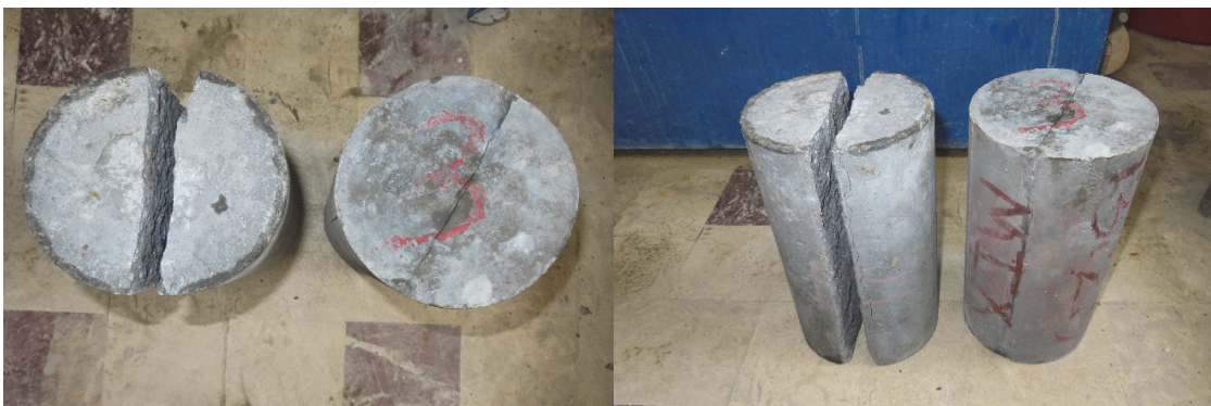
Figure 7: Tensile toughness of cylindrical samples.
