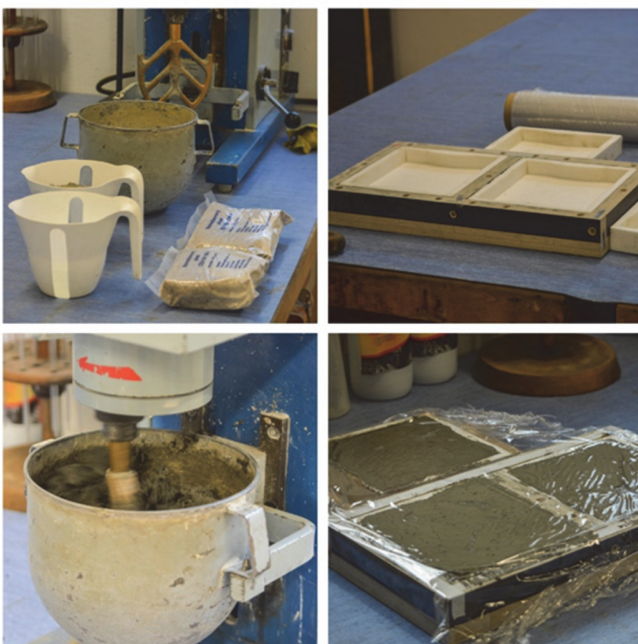
Figure 4: Specimens preparation in silicone molds installed in frames made of waterproof plywood.
