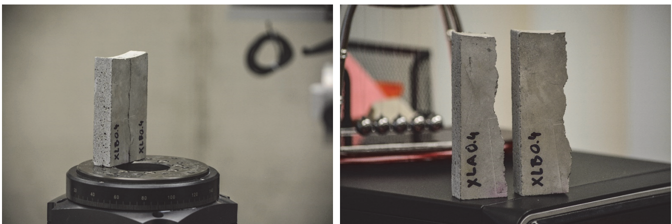
Figure 1: Parts of MCT specimens cut off for X-ray tomography.
