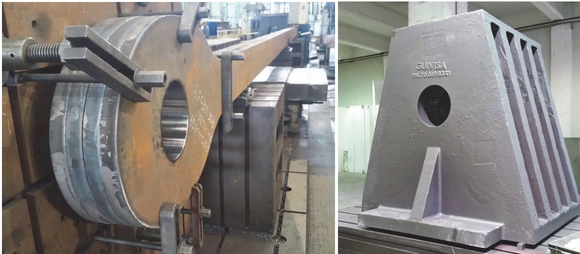
Figure 24: Eye-bar and saddles during manufacture process.
