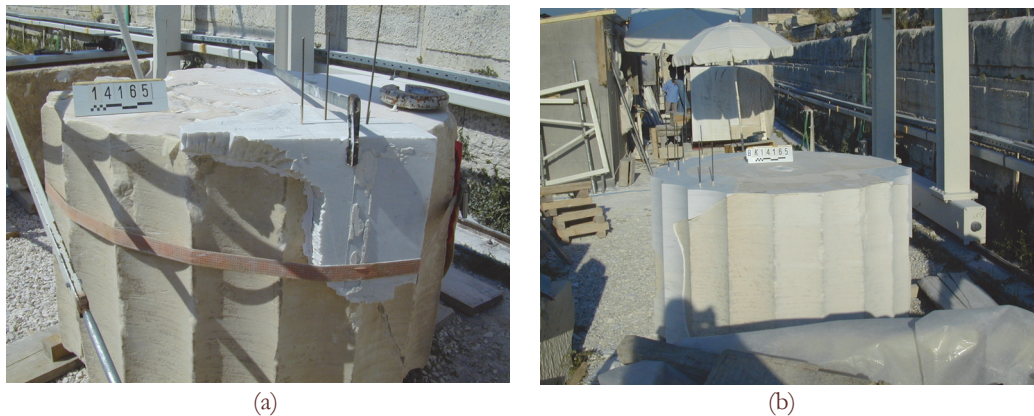
Figure 10: (a) Titanium bars were inserted from the upper side of the first supplement after its fitting with the rest volume of the drum. (b) Titanium bars were inserted from the upper side of the second supplement after its fitting with the rest volume of the drum.
