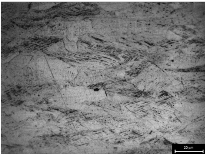
Figure 3. Strain induced martensite in steel A.
