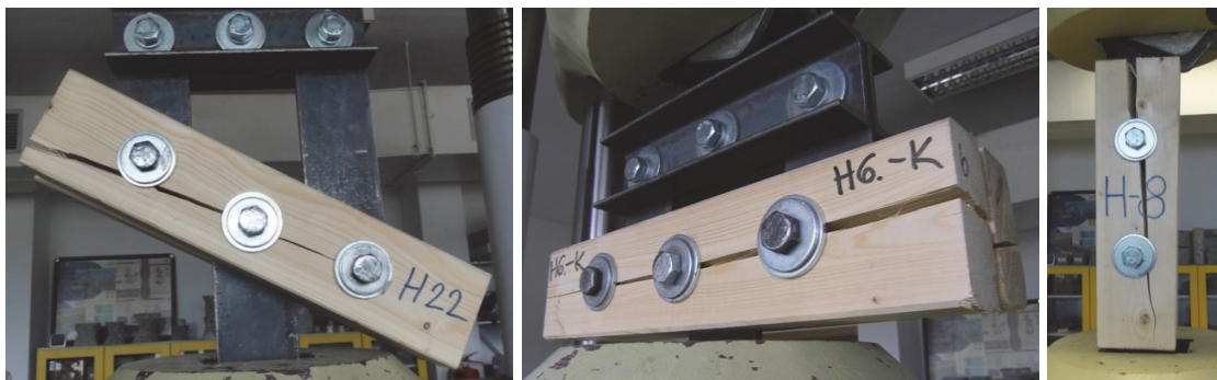
Figure 6: Damaged squared timber samples loaded in tension at different angles.
