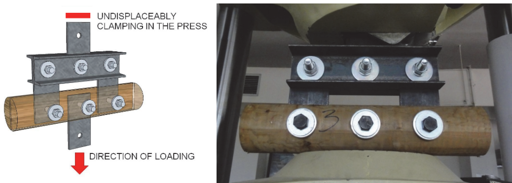
Figure 1: Steel product for testing in tension perpendicular to the grain and sample in press machine.
