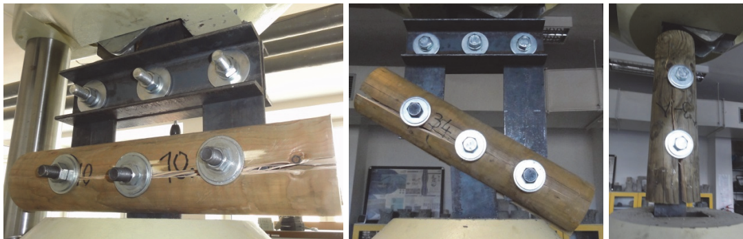
Figure 5: Damaged round timber samples loaded in tension at different angles.
