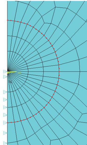
Figure 2c: Detail of the FE mesh for the ring 0.5 mm variant with nodal selection (red dots at the distance 0.5 mm from the crack tip).
