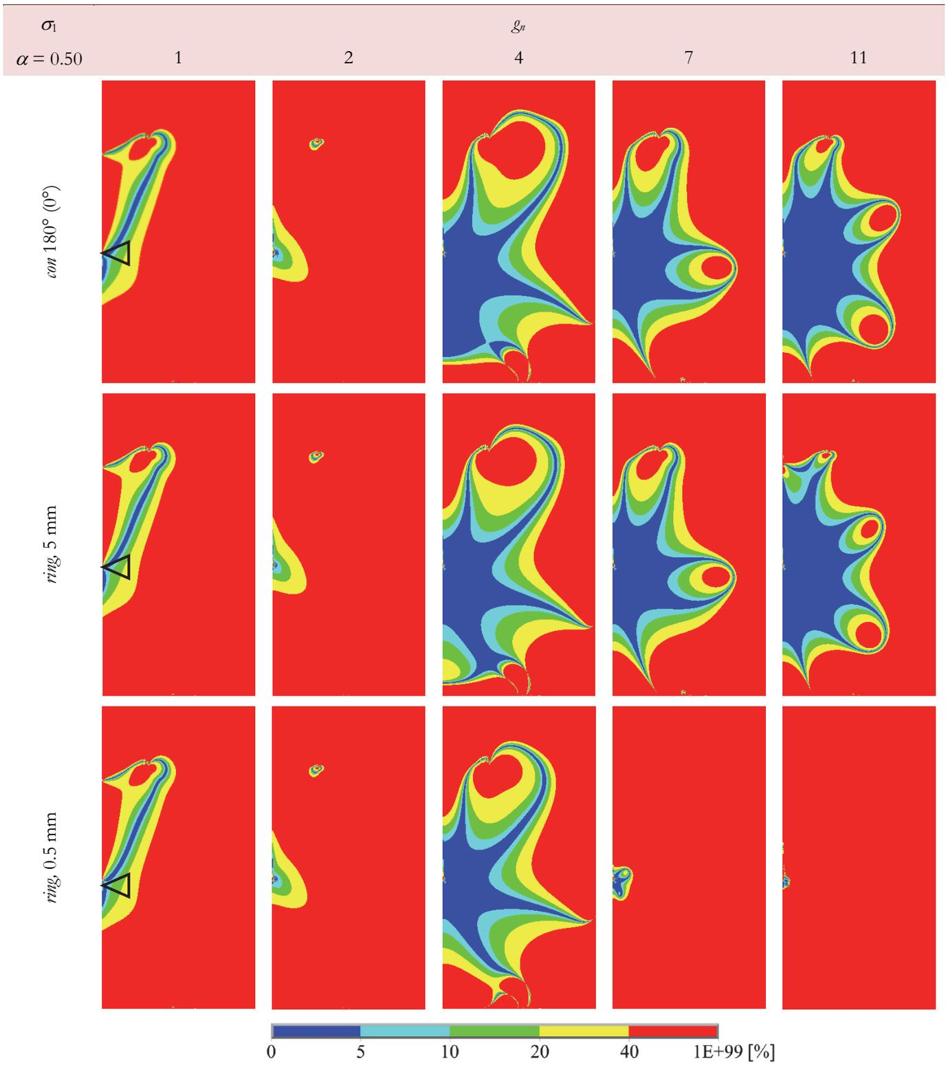
Figure 6: Relative error of principal tensile stress  $\sigma_1$  field approximation for chosen variants of nodal selection.
