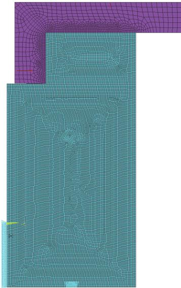
Figure 3a: Numerical model of the WST specimen, used finite element mesh [22].
