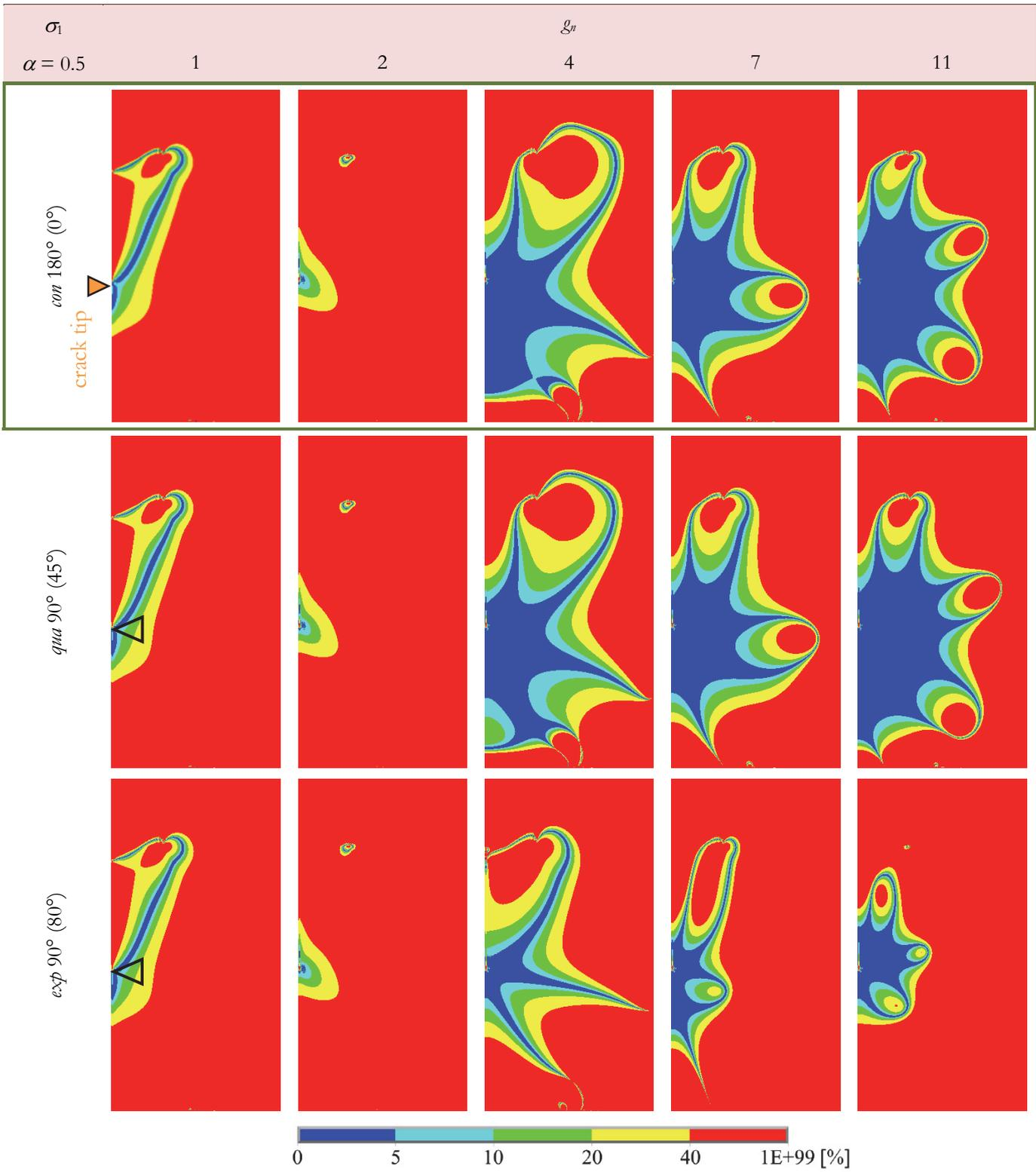
Figure 4: Relative error of principal tensile stress  $\sigma_1$  field approximation for chosen variants of nodal selection.
