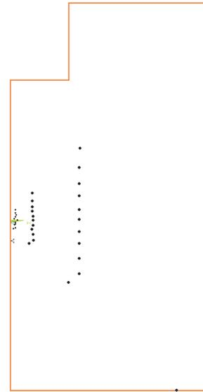
Figure 3c: Distribution of FE nodes for *qua* 90° (45°) variant of nodal selection [22].
