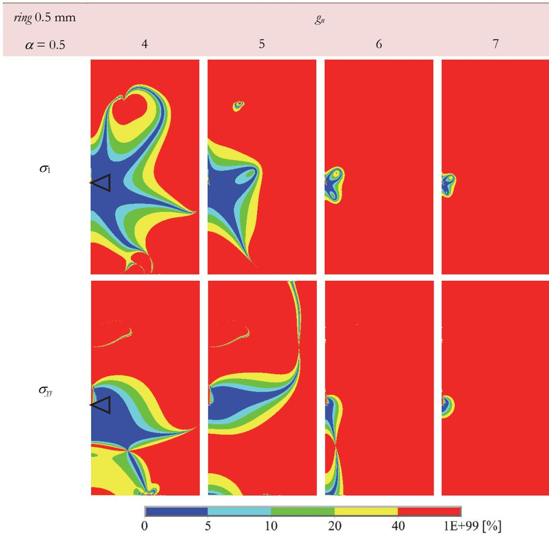
Figure 8: Progress of relative error of the  $\sigma_1$  and  $\sigma_y$  reconstruction with increasing number of Williams series terms used.
