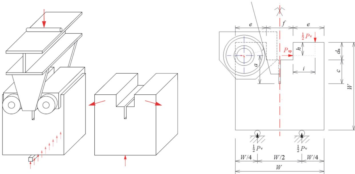
Figure 1: Wedge splitting test with the schema of loading imposition (left); geometry of the analysed wedge splitting test specimen (right)[15].
