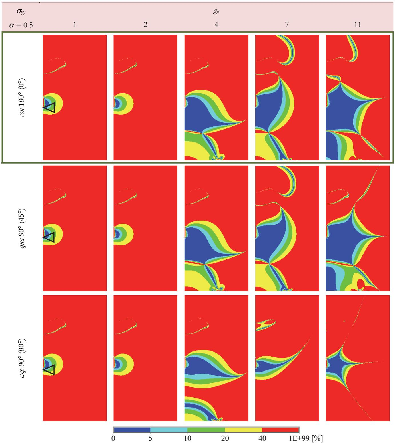
Figure 5: Relative error of crack opening stress  $\sigma_{yy}$  field approximation for chosen variants of nodal selection.
