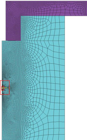
Figure 2a: Numerical model of the wedge splitting test, finite element mesh.
