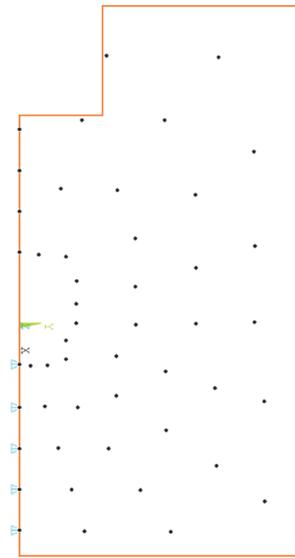
Figure 3b: Distribution of FE nodes for *con* 180° (0°) variant of nodal selection [22].
