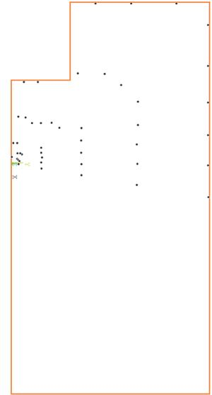
Figure 3d: Distribution of FE nodes for *exp* 90° (80°) variant of nodal selection [22].
