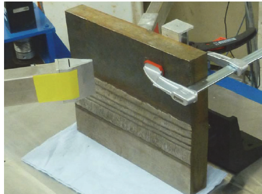
Figure 7: Section of Mock-up on diffractometer.
