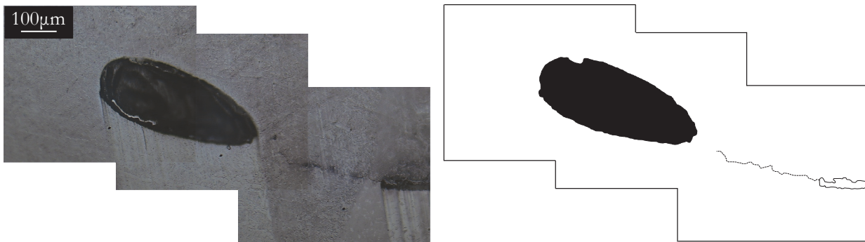
Figure 13: Crack propagation from tip of root region with welding defect.
