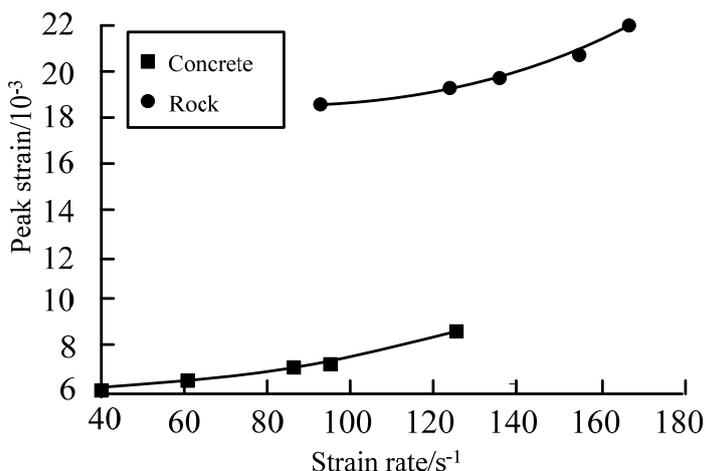
Figure 4: Correlation between peak strain and strain rate.
