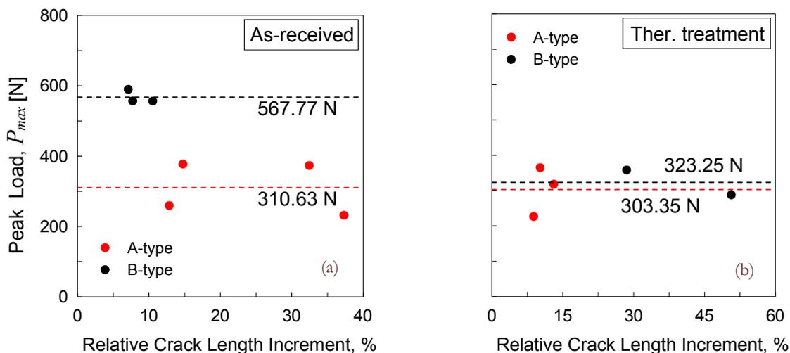
Figure 2: Peak load against relative crack length increment for: (a) the as-received and (b) the thermal pre-treated specimens.
