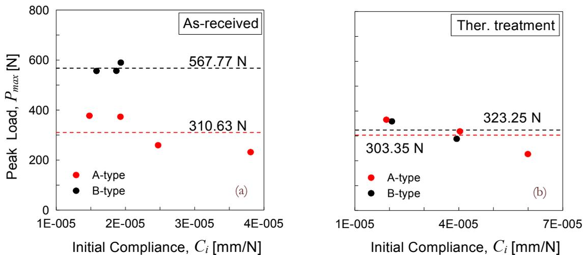
Figure 3: Peak load against initial compliance for: (a) the as-received and (b) the thermal pre-treated specimens.
