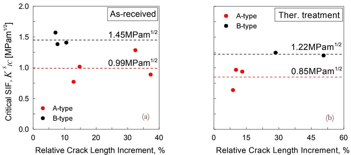
Figure 4: Critical SIF against relative crack length increment for: (a) the as-received and (b) the thermal pre-treated specimens.
