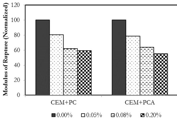
Figure 6: Modulus of rupture of cement composites with PC & PCA particles inclusions.
