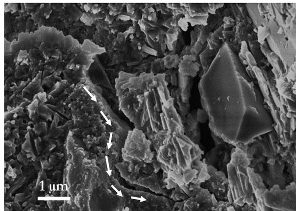
Figure 12: Crack propagation in cement composite matrix.
