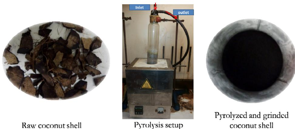
Figure 1: Synthesis of micro carbonized particles from coconut shell by pyrolysis
