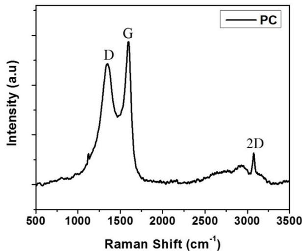
Figure 4: Raman spectroscopy of pyrolyzed coconut shell particles.
