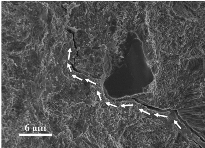
Figure 10: Crack contouring around a pyrolyzed coconut shells particles inclusion.
