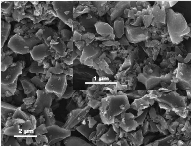
Figure 2: FESEM micrographs of pyrolyzed coconut shells particles.
