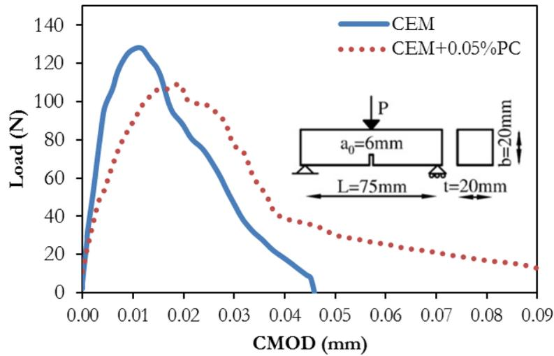
Figure 5: Typical load-CMOD curves for cement composites with and without pyrolyzed coconut shells particles.
