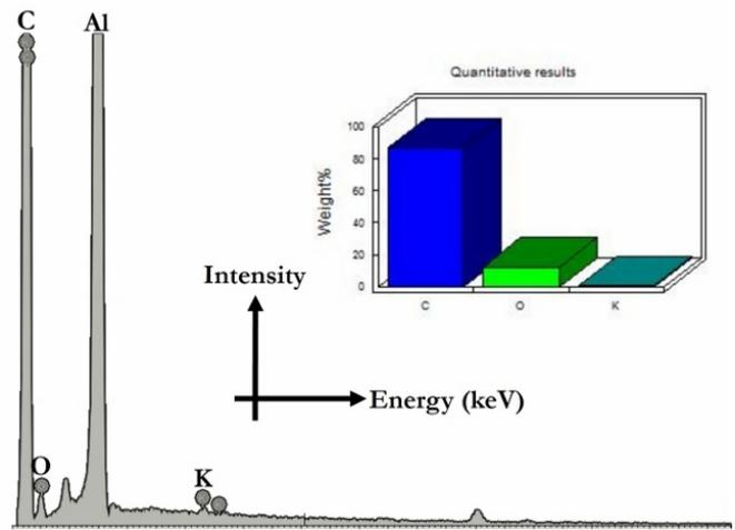
Figure 3: EDX analysis of pyrolyzed and ground coconut shells particles.
