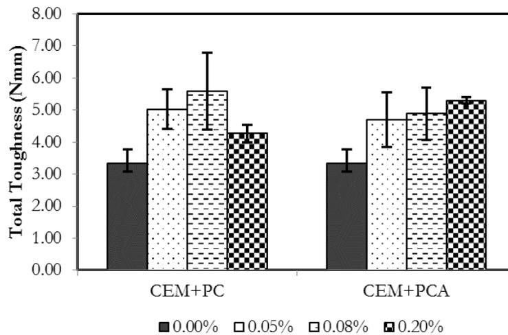
Figure 8: Toughness of the cement composites samples with various amounts of PC & PCA particles inclusions.
