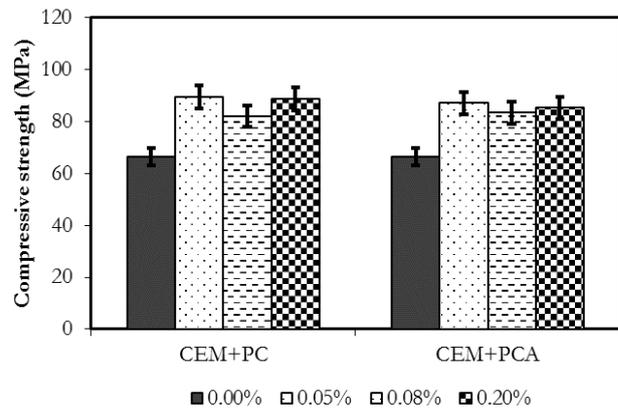
Figure 7: Compressive strength of the cement composites with PC & PCA particles inclusions.
