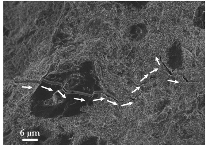
Figure 11: Crack passing through a large inert particle and crack branching.
