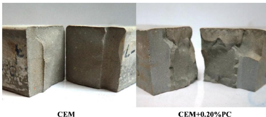
Figure 9: Typical fracture surfaces of the cement composites tested in flexure
