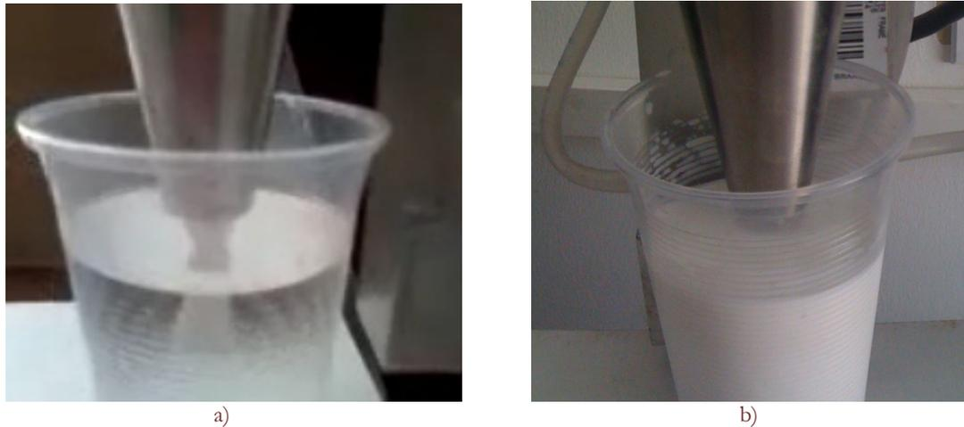
Figure 4: Ultrasonic fatigue testing of polymer ABS immersed in water a) and in oil b). No cavitation effect was observed during ultrasonic fatigue testing with specimens immersed in water or in oil.
