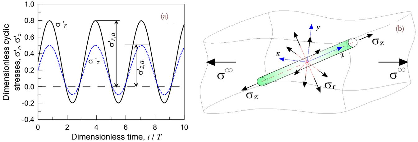
Figure 2: (a) Radial and axial cyclic dimensionless stresses vs time: definition of the effective stress amplitudes. (b) Scheme of the radial and axial matrix stresses near a cylindrical fibre.
