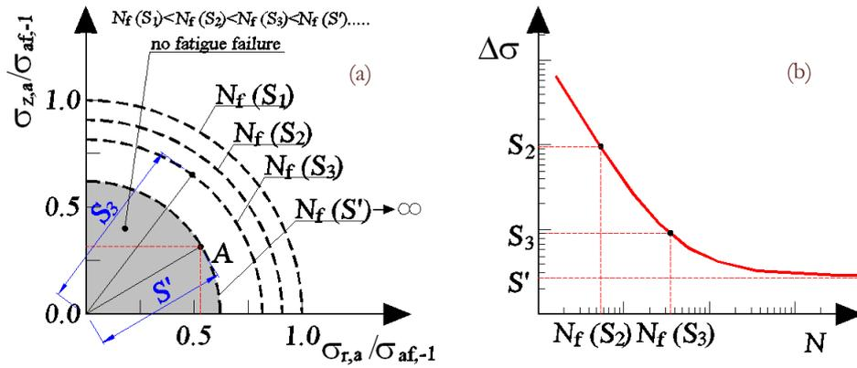
Figure 3: (a)  $\sigma_z - \sigma_r$  fatigue domains that identifies conventional fatigue life for a biaxial normal stress state. (b) The Wöhler curve for a uniaxial cyclic stress history.
