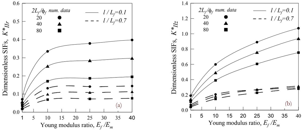
Figure 4: Dimensionless radial and longitudinal Mode II SIF, (a)  $K_{II,r}$  and (b)  $K_{II,z}$ , vs Young modulus ratio,  $E_f/E_m$ , for different values of fibre aspect ratio,  $2 \cdot L_f/\phi_f$ , and relative debonded length equal to 0.1 and 0.7.
