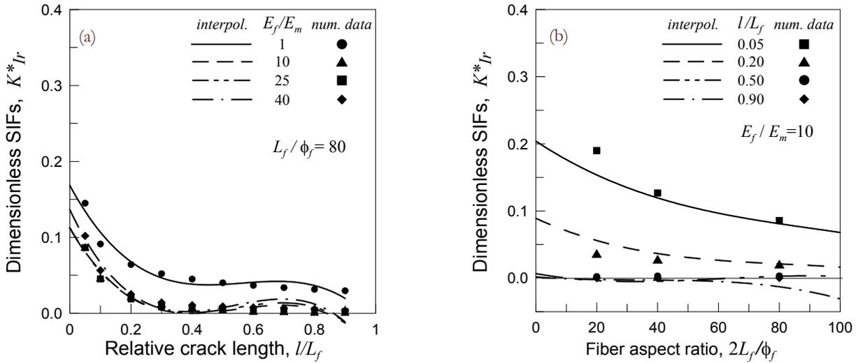
Figure 5: Dimensionless radial and longitudinal Mode II SIF, (a)  $K_{II,r}$  and (b)  $K_{II,z}$ , vs Relative crack length,  $l/L_f$ , for different values of fibre aspect ratio,  $2 \cdot L_f/\phi_f$ , and relative debonded length equal to 0.1 and 0.7.
