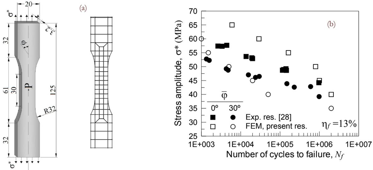
Figure 6: (a) Geometrical dimensions, expressed in (mm), and FEM model of the specimen; (b) the Wöhler curves of the glass fibre-reinforced polyamide specimen: experimental [28] and present results.
