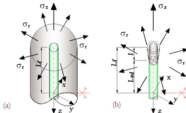
Figure 1: (a) Cylindrical fibre surrounded by a cylindrical portion of matrix material; (b) partially detached fibre under radial and axial stresses.
