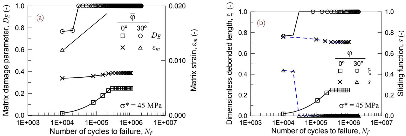
Figure 7: (a) Damage and strain evolution in the matrix (at point P) vs the number of stress cycles; (b) dimensionless fibre debonded length  $\xi$ , and sliding parameter  $s$ , (at point P) vs the number of stress cycles.
