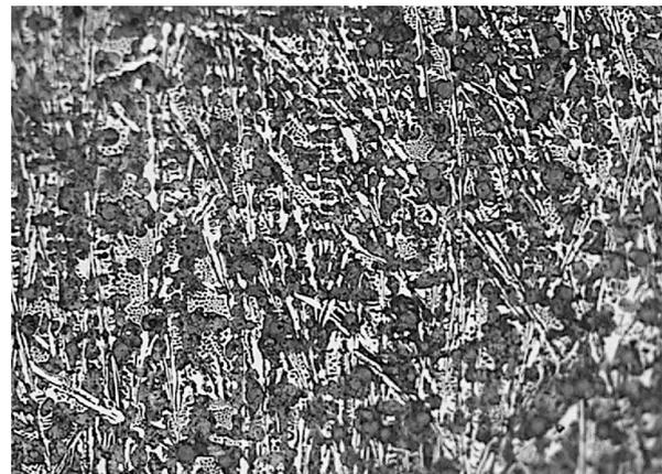
Figure 4: Defects in DCIs. Carbides (x200). Courtesy of Zanardi Fonderie S.p.A.
