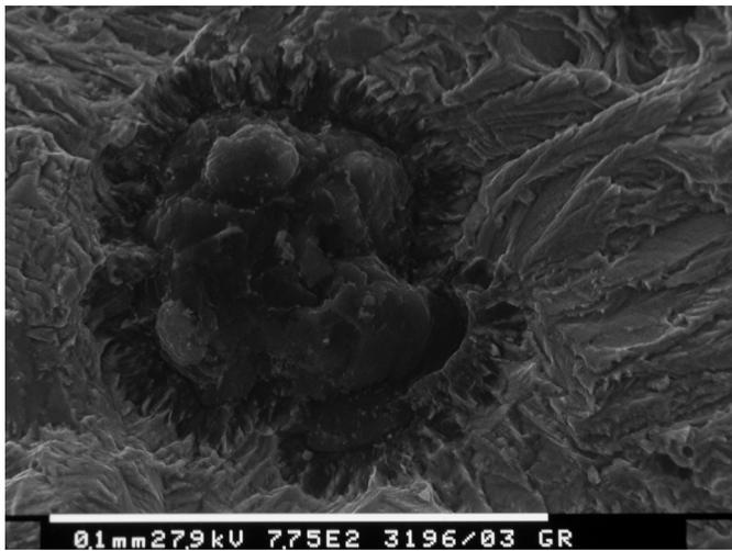
Figure 14: Ferritized DCI. SEM fracture surface analysis ( $\Delta K = 12 \text{ MPa}\sqrt{\text{m}}$ ).
