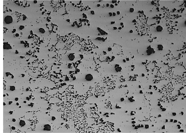
Figure 2: Defects in DCIs. Chunky graphite (x200). Courtesy of Zanardi Fonderie S.p.A.
