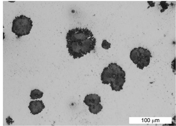
Figure 8: Pearlitic DCI after long annealing heat treatment (ferritic matrix and degenerated graphite elements).
