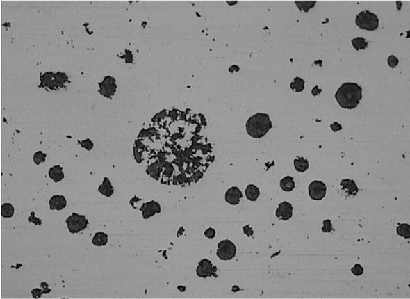
Figure 1: Defects in DCIs. Exploded graphite (x200). Courtesy of Zanardi Fonderie S.p.A.
