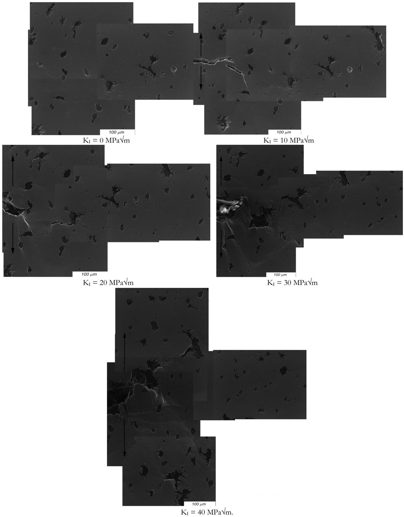
Figure 18: Overloads effect on fatigue crack (arrows shows the loading direction).
