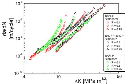
Figure 11: Matrix and loading conditions influence on DCIs ferritic-pearlitic fatigue crack propagation resistance [6].
