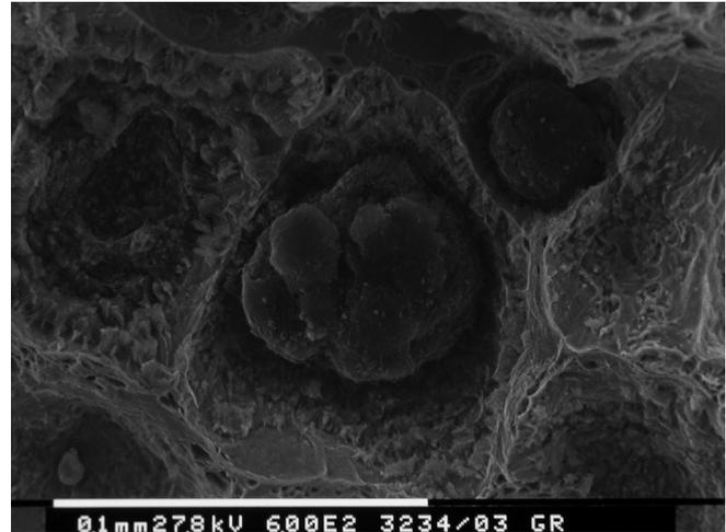
Figure 20: SEM observation of the fracture surface (after overloads).
