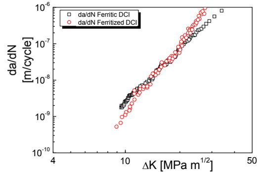
Figure 12: Degenerated graphite elements influence on fatigue crack propagation in ferritic DCI.
