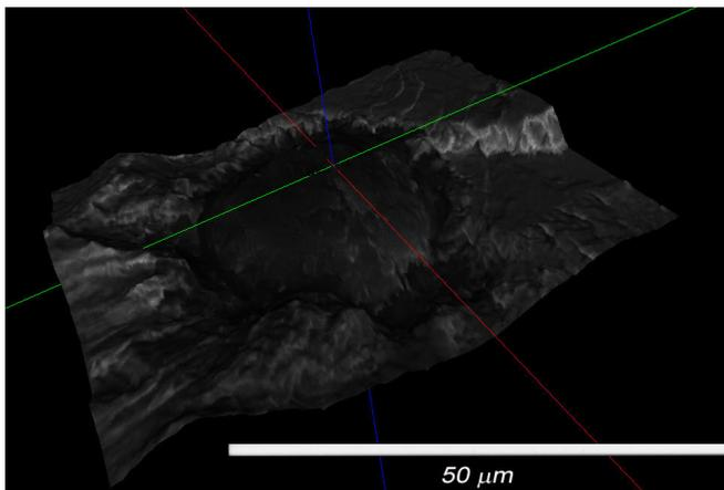
Figure 16: Ferritized DCI. SEM fracture surface analysis: 3D reconstruction ( $\Delta K = 14 \text{ MPa}\sqrt{\text{m}}$ ).
