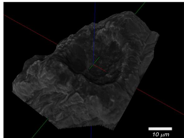
Figure 17: Ferritized DCI. SEM fracture surface analysis: 3D reconstruction ( $\Delta K = 15 \text{ MPa}\sqrt{\text{m}}$ ).
