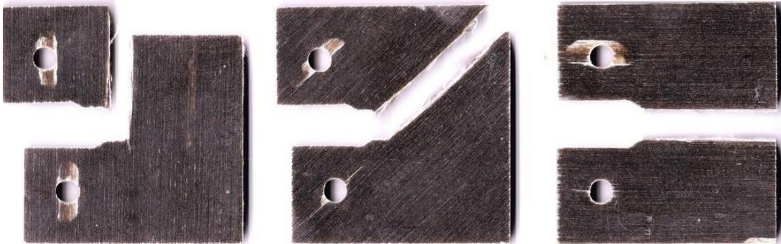
Figure 5: Compact tension specimens with different directions after cyclic loading (fibre volume fraction 35%).
