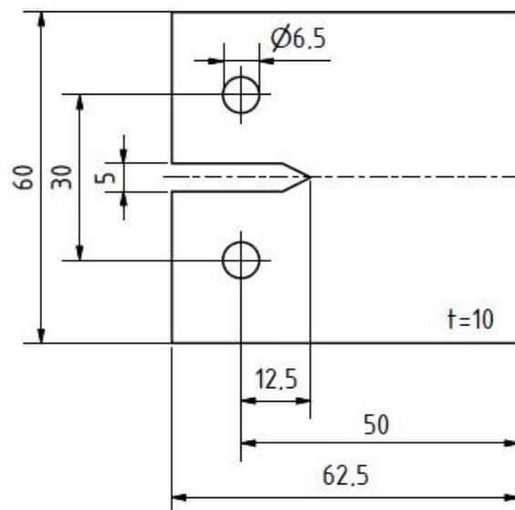
Figure 2: Geometric dimensions of the investigated compact tension specimen (dimensions in mm).
