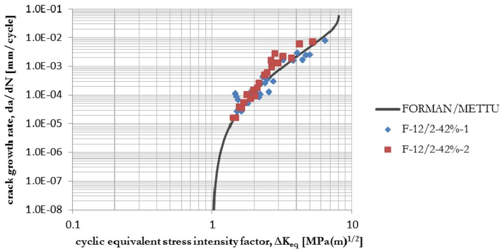
Figure 7: Fatigue crack growth rate data for compact tension specimens (90° fibre direction, R = 0.1).
