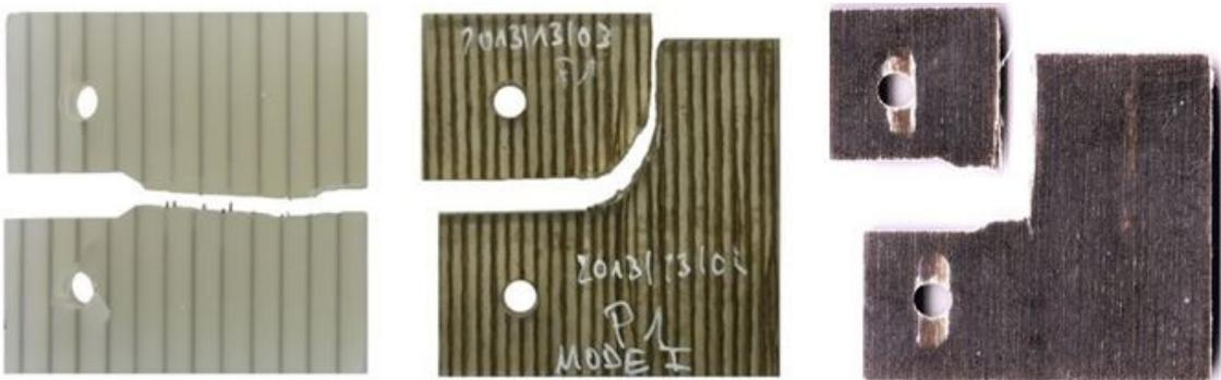
Figure 6: Compact tension specimens with different fibre volume fractions (0° fibre direction).
