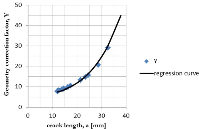
Figure 10: Geometry correction factor data for compact tension specimen ( $90^\circ$  fibre direction).
