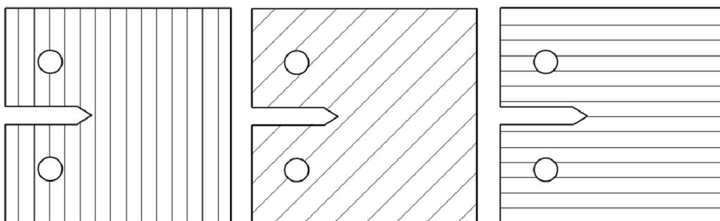
Figure 4: Schematic illustration of compact tension specimens with different fibre directions (0°, 45°, 90°).
