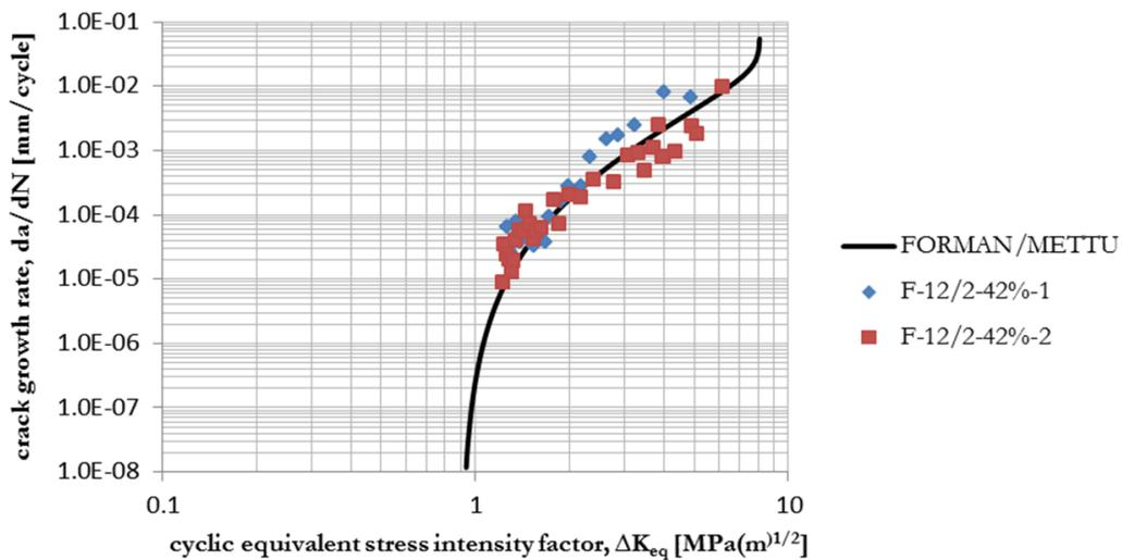
Figure 8: Fatigue crack growth rate data for compact tension specimens (45° fibre direction, R = 0.1).
