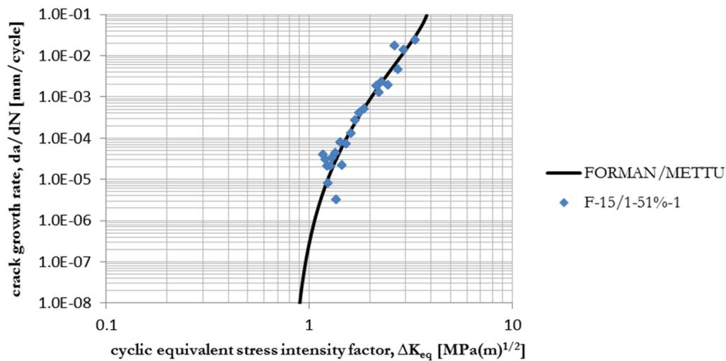
Figure 9: Fatigue crack growth rate data for compact tension specimen (0° fibre direction, R = 0.1).
