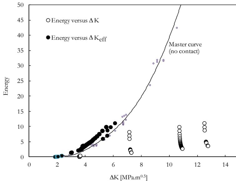
Figure 6: Effect of effective stress intensity factor range,  $\Delta K_{eff}$ , on dissipated energy after overloads.
