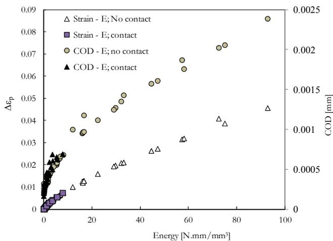
Figure 5: Crack opening displacement versus energy and plastic strain range versus energy.
