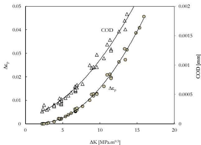
Figure 2: Effect of  $\Delta K$  on range of plastic strain and crack opening displacement (no contact).
