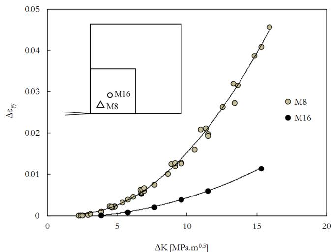
Figure 4: Effect of mesh on plastic strain range.
