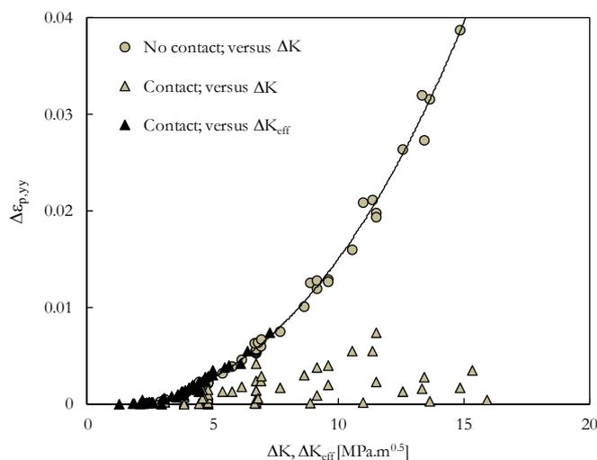
Figure 3: Effect of effective stress intensity factor range,  $\Delta K_{eff}$ , on plastic strain range.
