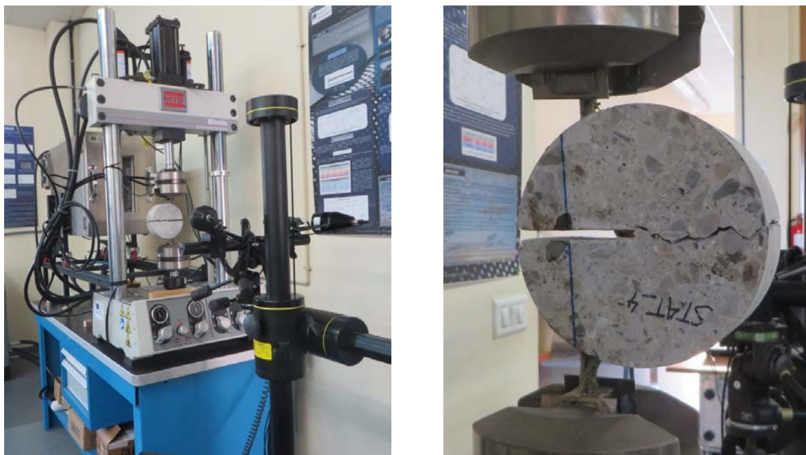
Figure 3: Specimen set up into the servohydraulic MTS Bionix 25 kN machine.
