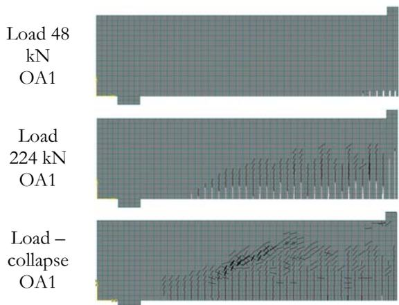
Figure 4: Failure in a beam, OA1.
