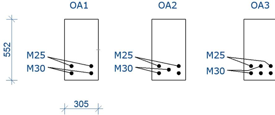
Figure 2: Cross-section of the beams.
