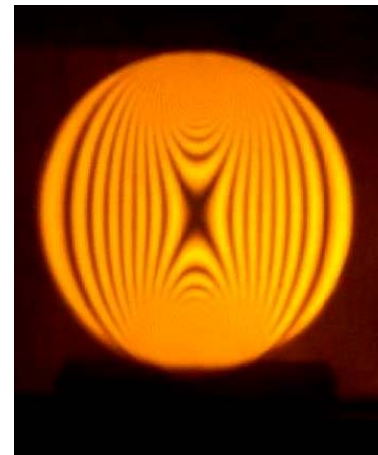
Figure 5. Isochromatic fringes in calibration disk.
