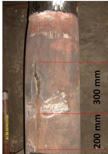
Figure 5: Determination of damage by visual inspection.
