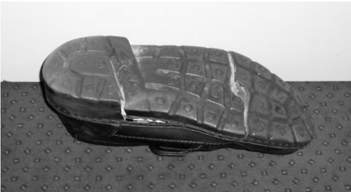
Figure 18. Cracks in sole of walking shoe.
