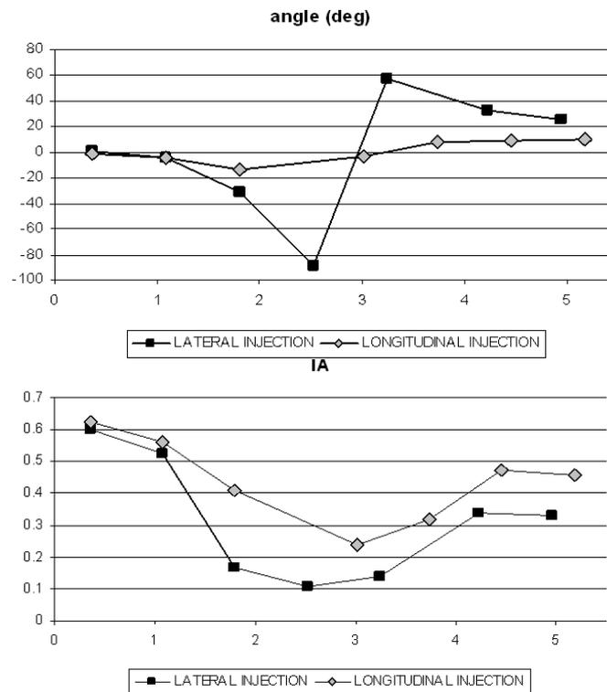
Figure 4: Preferred fibre orientation with respect to specimen y axis (above), and Index of Anisotropy IA (below), at different z positions (mm), core layer.
