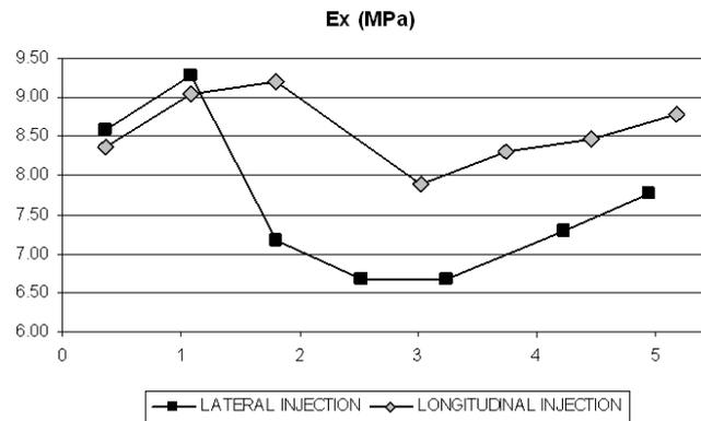
Figure 5: Apparent elastic modulus (MPa) along specimen x axis, at different z positions (mm), core layer.
