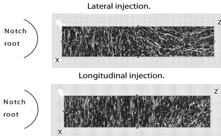
Figure 3: Lateral and longitudinal injection, point A, core layer:  $\mu$ -CT reconstruction.
