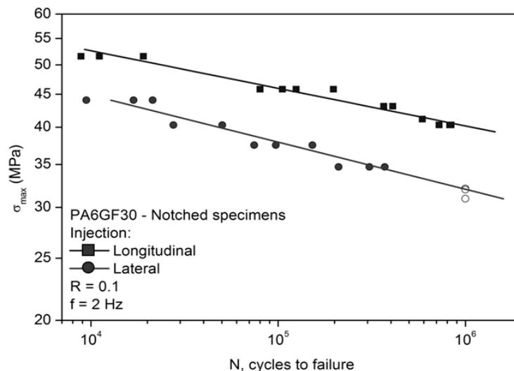
Figure 2: S-N curves for specimens with lateral notches.
