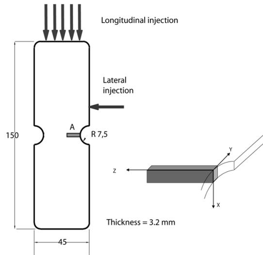
Figure 1: Specimens type, dimensions and injection gates; position of micro-CT examined samples.
