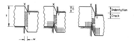
Figure 2 Single shear plane model of cropping showing flow, and flow and fracture  $\frac{1}{2}$
