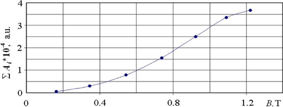
Fig. 3. The effect of the amplitude value of magnetization in the plate/strip on the total sum of amplitudes of the MAE signal impulses.
