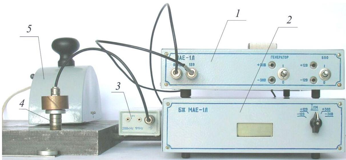
Fig. 6. A photograph of the system MAE-1L: 1 – the main unit, 2 – battery power unit, 3 – preamplifier, 4 – piezoceramic transducer, 5 – electromagnet.
