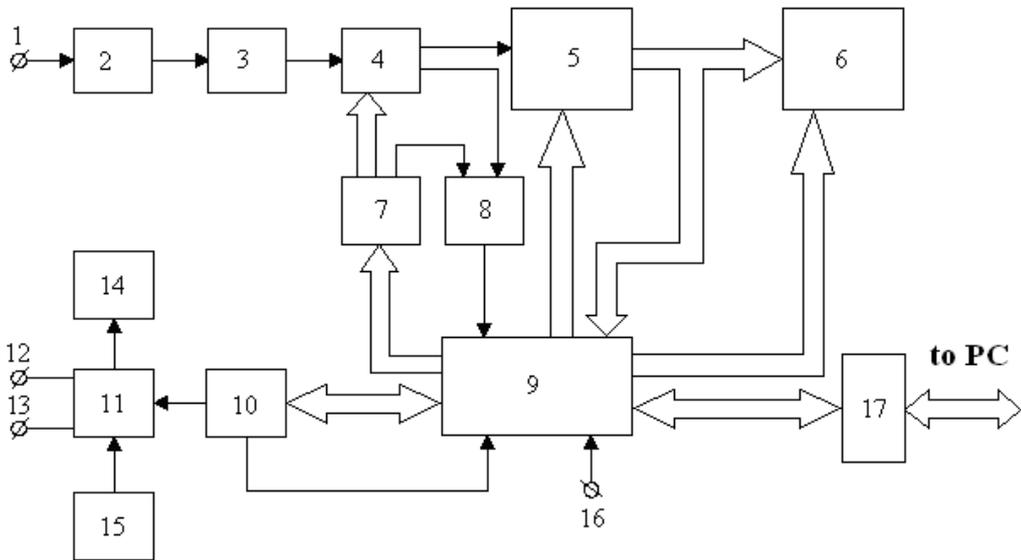
Fig. 5. Block diagram of a PC-operated system for acquisition, processing and logging of MAE signals.
