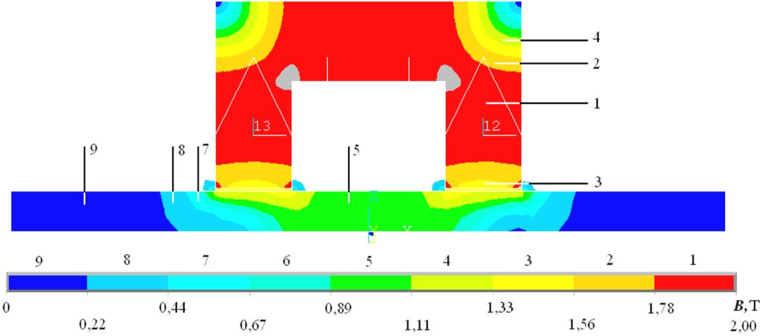
Fig. 4. Longitudinal section of the plate and the core of electromagnet with distribution of the amplitude of magnetization in ferromagnetic materials.
