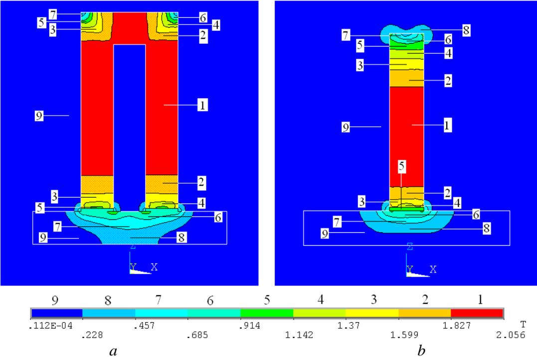
Fig. 1. Distribution of the magnitude of the magnetization vector in the plane XOZ: *a* – for the U-type electromagnet and *b* – for the I-type electromagnet.
