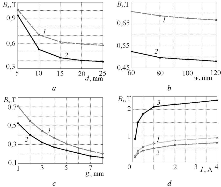
Fig. 2. Dependencies of the  $B_x$  component of the magnetization vector along the  $OZ$  axis for the U-type electromagnet on the thickness  $d$  of the sample (a), its width  $w$  (b), thickness of the air gap  $g$  (c), and the magnetizing current  $I$  (d): at 1 mm depth – graph 1; at 4 mm depth – graph 2; in the core of electromagnet – graph 3.
