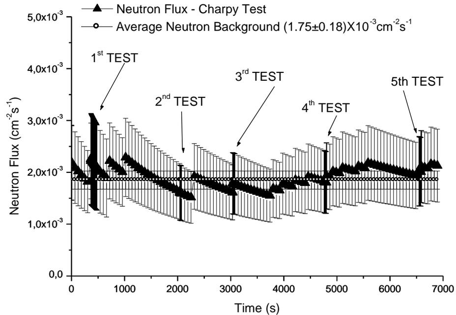
Fig.5. Diagram of the Atomtex neutron acquisition during the Charpy tests.
