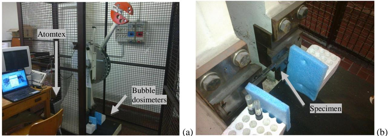
Fig.4. View of the Charpy pendulum, with indication of the sensors position (a); detail of the BDT sensors positioning beside the specimen (b).
