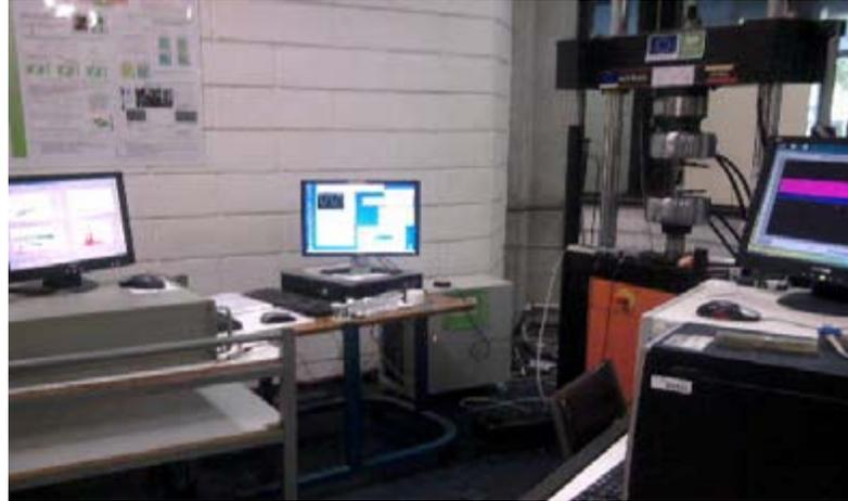
Fig.2. Machine and instrumentation for fatigue tests.
