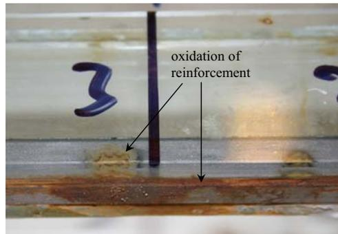
Figures 9 and 10: Salt deposition and oxidation of reinforcement after 8 weeks of salt-water-spraying
