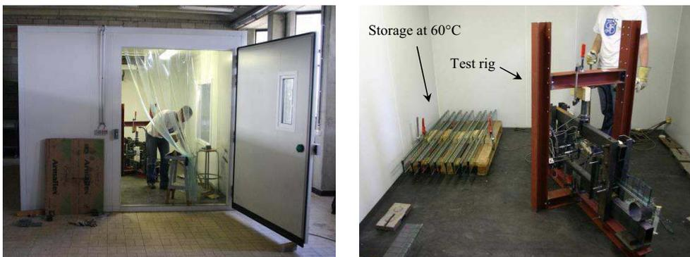
Figures 3 and 4: Beam specimens stored and tested at 60°C in a climatic room.
