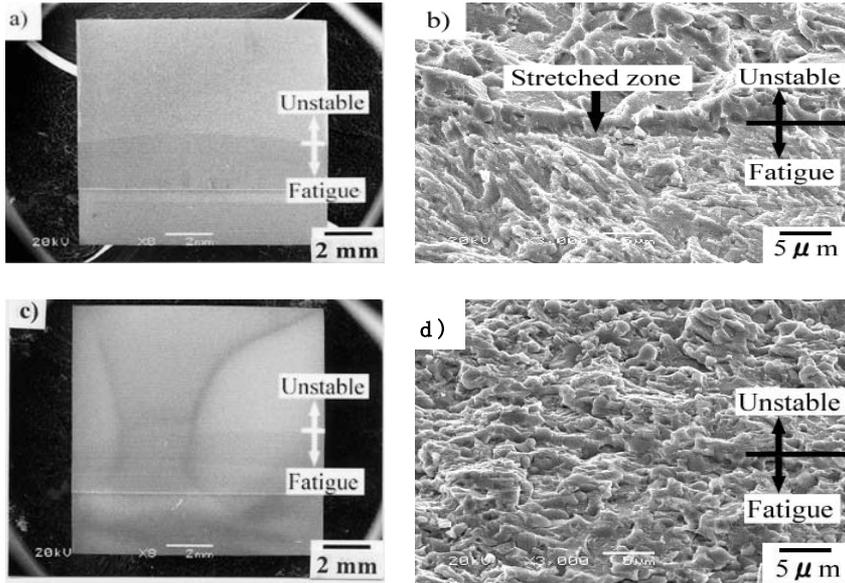
Fig.6 Stretched zone on three point bending fracture surface.
