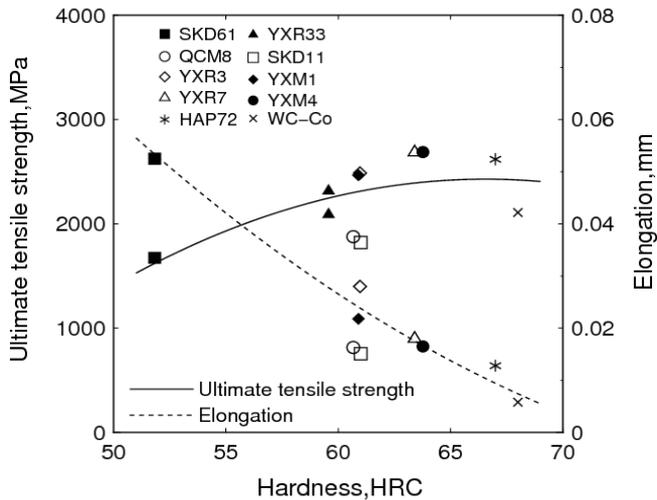
Fig.1 Relation among ultimate tensile strength, elongation and Rockwell C scale hardness number of cold forging die steels.
