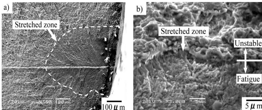
Fig.8 Fracture surface of cold forging die.
