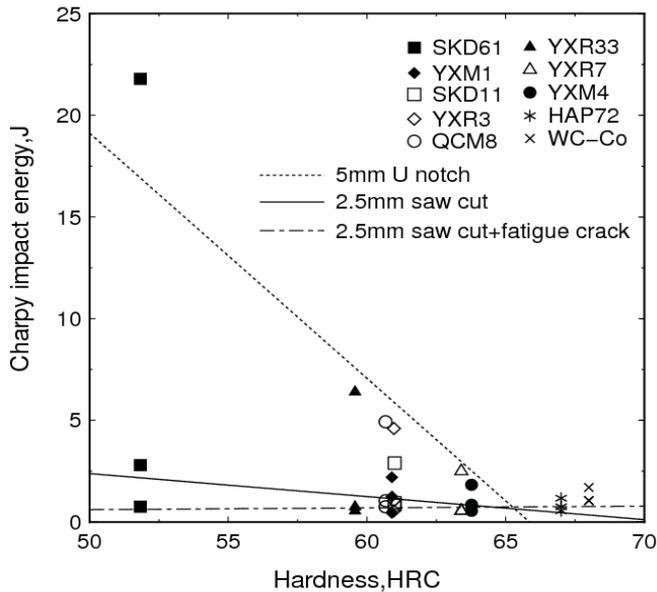
Fig.2 Charpy impact energy of cold forging die steels with different notch figure.
