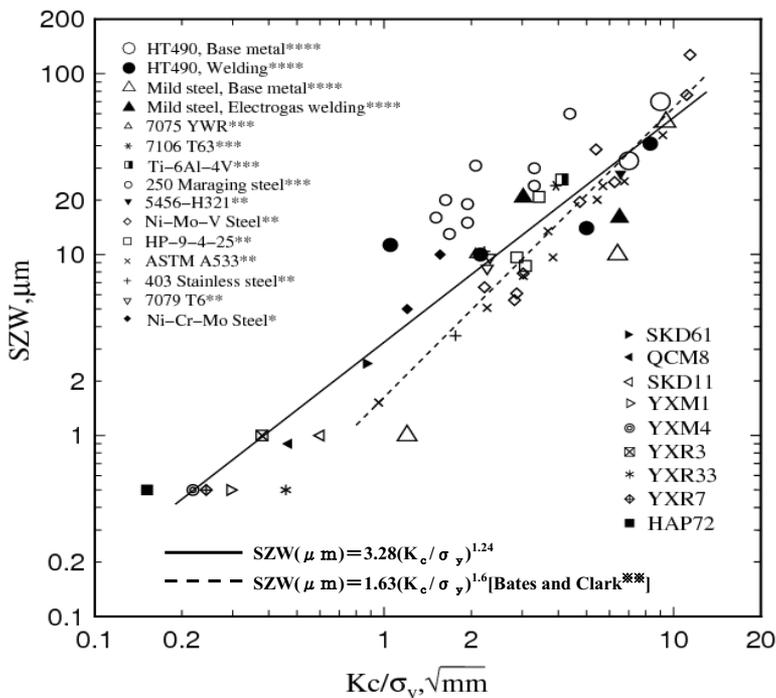
Fig.7 Stretched zone width as a function of  $K_c / \sigma_y$ .
