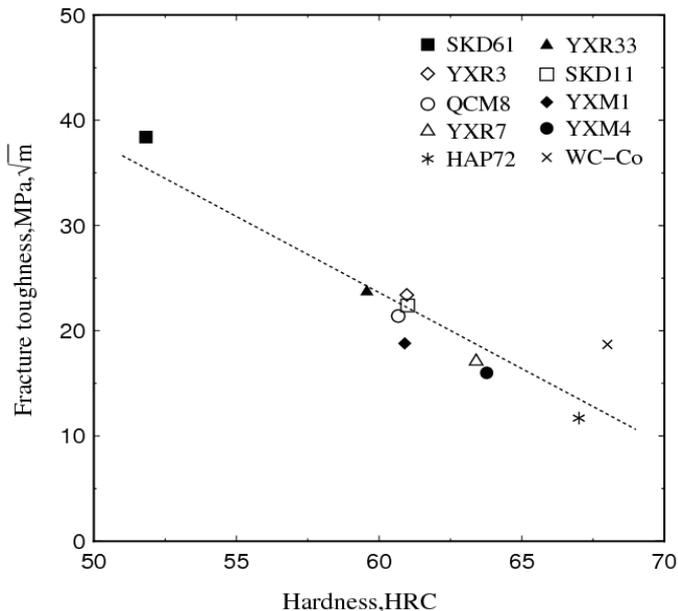
Fig.3 Relation between fracture toughness and hardness of cold forging die steels.
