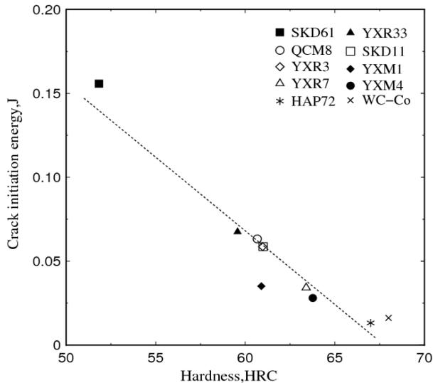
Fig.5 Crack initiation energy as a function of Rockwell C scale hardness number.
