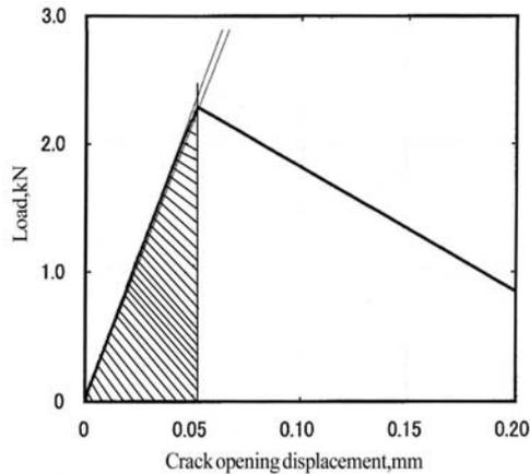
Fig.4 Relation between load and crack opening displacement.
