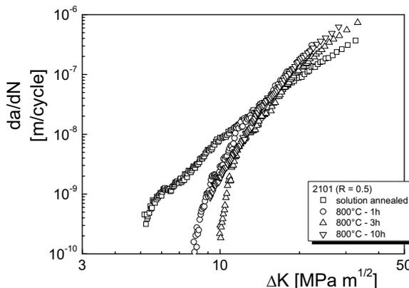
Fig. 7: 2101 “lean” DSS fatigue crack propagation resistance: heat treatment influence (R = 0.5).
