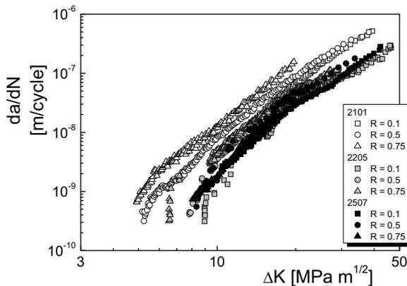
Fig. 2: Chemical composition influence on DSSs fatigue crack propagation resistance (solution annealed conditions).
