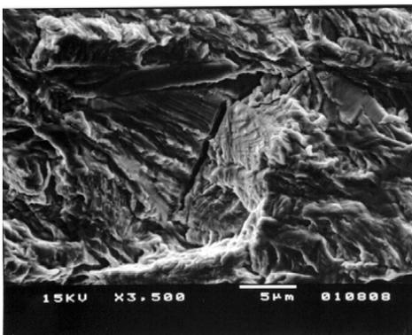
Fig. 3: Solution annealed 2205 DSS fracture surface ( $\Delta K = 15 \text{ MPa}\sqrt{\text{m}}$ ;  $R = 0.5$ ).
