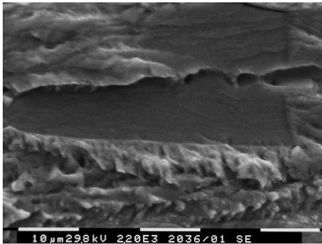
Fig. 5: Solution annealed 2101 “lean” DSS fracture surface ( $\Delta K = 6$  MPa√m; R = 0.5).
