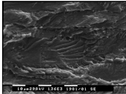
Fig. 6: Solution annealed 2101 “lean” DSS fracture surface ( $\Delta K = 11$  MPa√m; R = 0.1).
