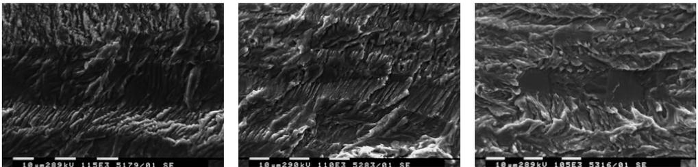
Fig. 10: 2101 DSS fracture surface analysis (threshold conditions). From left to right: 800°C - 1h; 800°C - 3h; 800°C - 10h.
