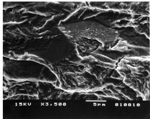
Figure 4: Solution annealed 2205 DSS fracture surface ( $\Delta K = 25 \text{ MPa}\sqrt{\text{m}}$ ;  $R = 0.5$ ).
