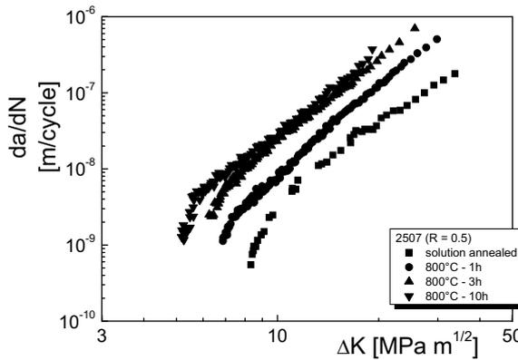
Fig. 9: 2507 “super” DSS fatigue crack propagation resistance: heat treatment influence (R = 0.5).
