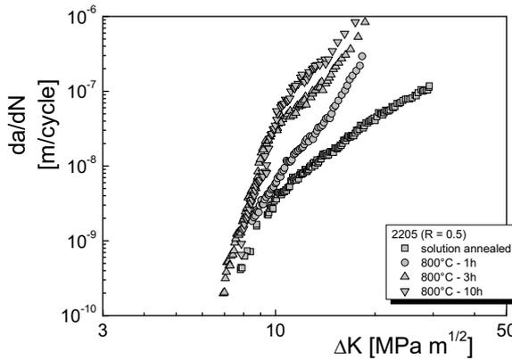
Fig. 8: 2205 “standard” DSS fatigue crack propagation resistance: heat treatment influence (R = 0.5).
