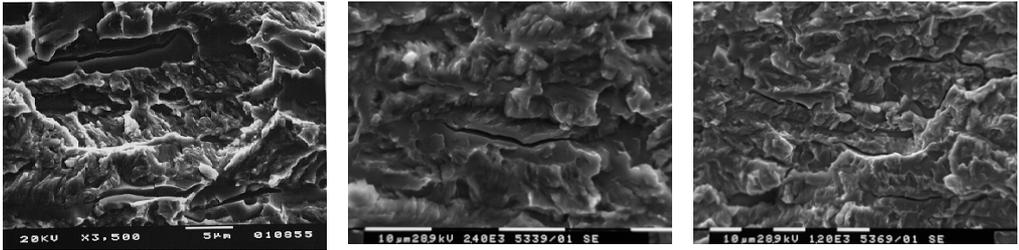
Fig. 11: 2205 DSS fracture surface analysis ( $\Delta K = 12 \text{ MPa}\sqrt{\text{m}}$ ;  $R = 0.5$ ). From left to right: 800°C - 1h; 800°C - 3h; 800°C - 10h.
