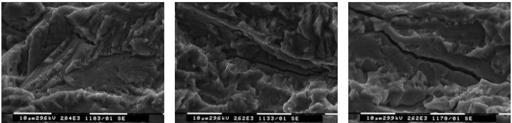
Fig. 12: 2507 DSS fracture surface analysis ( $\Delta K = 12 \text{ MPa}\sqrt{\text{m}}$ ;  $R = 0.5$ ). From left to right: 800°C - 1h; 800°C - 3h; 800°C - 10h.
