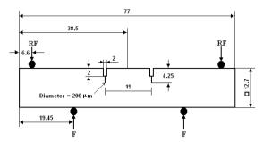
Fig. 1. Four point double-notch bend specimens.
