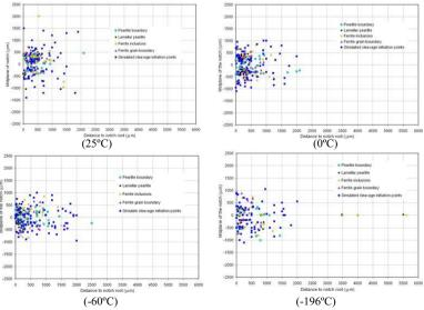
Fig. 5. Experimental and CAFE correlation of initiation points at -60°C.
