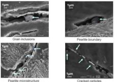
Fig. 2. Four cleavage fracture nucleation micromechanisms.
