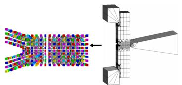
Fig. 6. Charpy test and the CA arrays created in the damage region.
