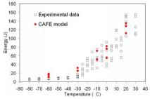
Fig. 8. CAFE simulation of the ductile-brittle transition.
