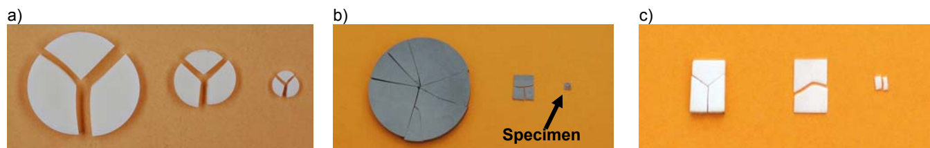
Fig. 4: Fractured B3B test specimens: a) discs of alumina specimens having a different size, b) silicon nitride specimen; the number of pieces, in which the specimen breaks, increases with the stored elastic energy and c) rectangular plate specimens made of zirconia ceramic.
