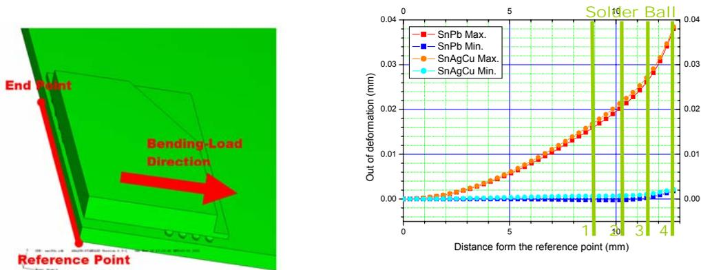
Figure 15. Out-of-plane deformation along to the transverse direction.
