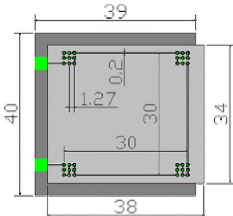
Figure 3. Dimensions of thermal specimen type #1 (mm).
