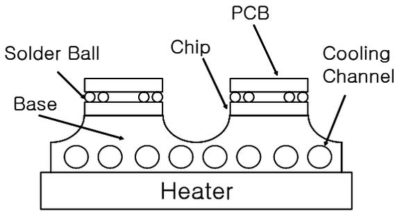
Figure 1. A schematic view of pseudo power cycling machine
