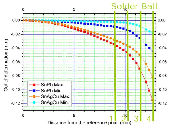
Figure 14. Out-of-plane deformation along to the bending-load direction.
