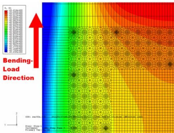
Figure 12. Out-of-plan deformation of PWB under PBGA package during thermal cycling tests.
