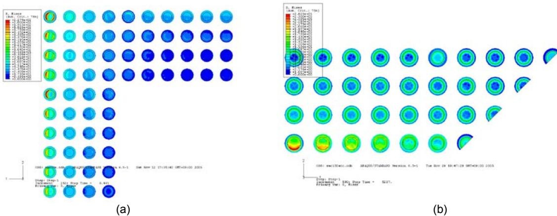
Figure 17. The applied stress distribution on the solder balls at bending and thermal cycling tests. (a) bottom view of solder balls in SnAgCu 50N bending cycling case (b) view of solder ball in SnAgCu 30~150°C thermal cycling case
