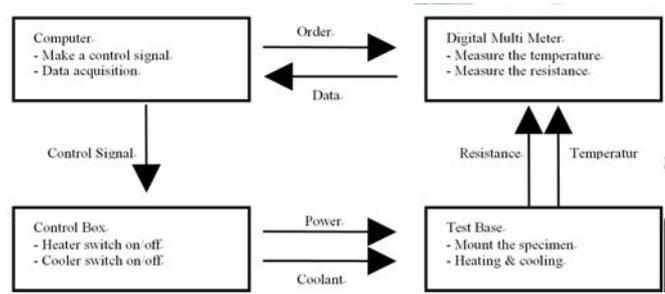
Figure 2. System flow chart of pseudo power cycling machine
