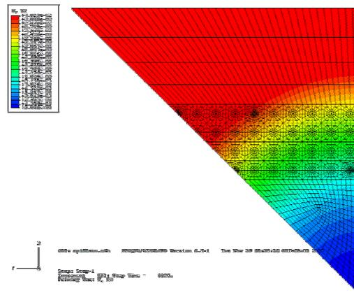
Figure 13. Out-of-plan deformation of PWB under PBGA package during bending cycling tests.
