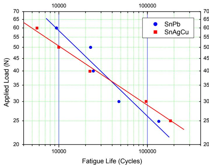
Figure 11. Maximum applied bending load vs. fatigue life curve
