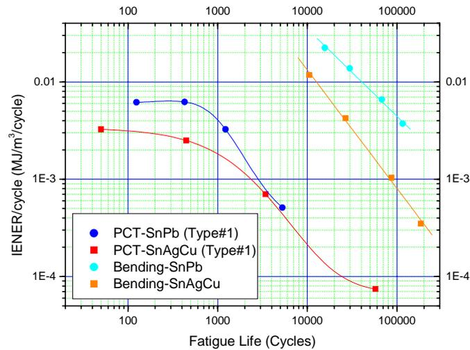
Figure 20. The inelastic dissipation energy versus fatigue life curve
