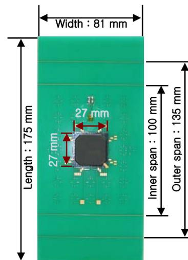
Figure 6. Four point bending test specimen, 256PBGA package was attached to the PWB board
