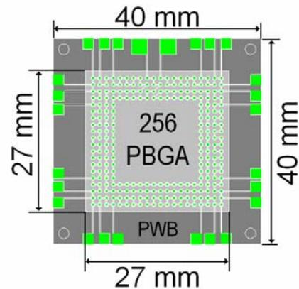
Figure 4. Dimensions of thermal specimen type #2 (mm).
