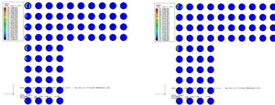
Figure 18. The creep and plastic energy density of solder joints' bottom area during a bending cycling test
