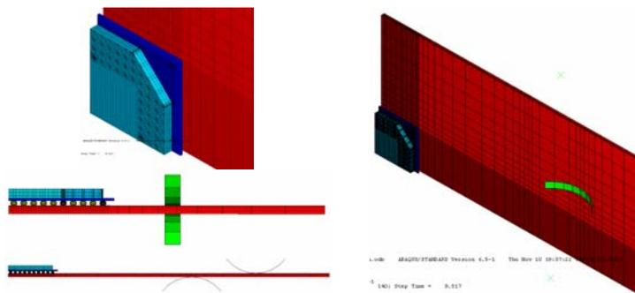
Figure 9. Finite element model for the bending cycling specimen
