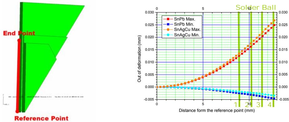
Figure 16. Out-of-plane deformation in thermal cycling case (type #2).
