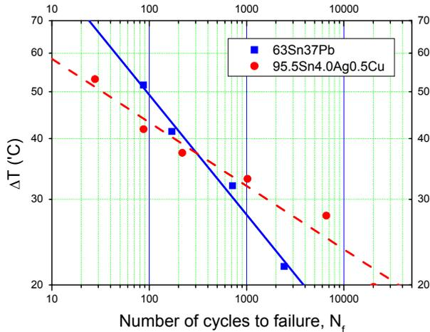
Figure 10. Maximum temperature difference between package and PWB vs. fatigue life curve
