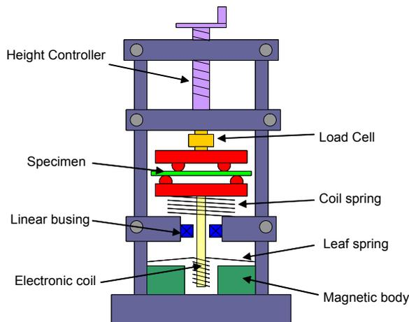
Figure 5. Mechanical bending test system using an electro-magnetic coil.
