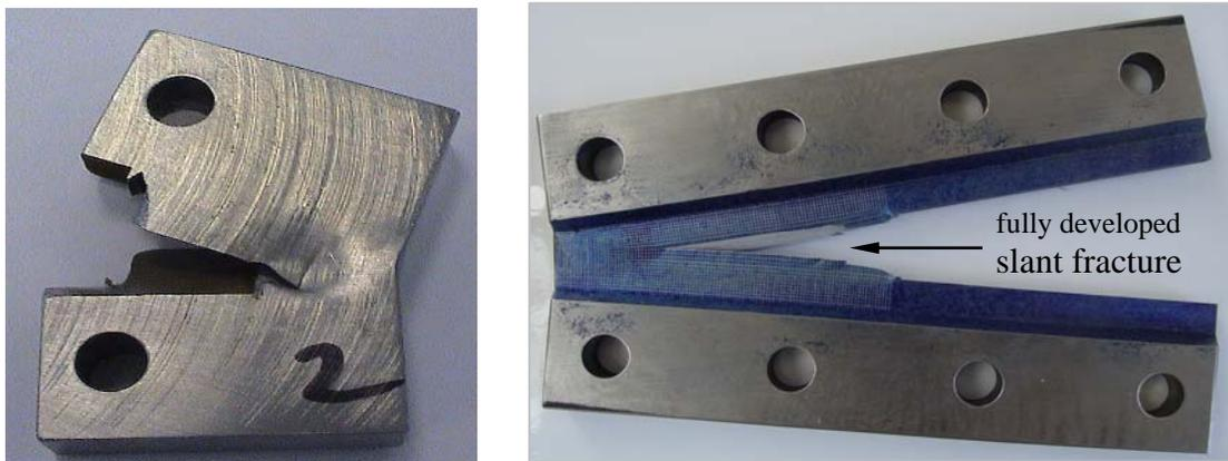
FIGURE 2. Photograph of slant notch C(T) (left) and modified DCB (right) after the test
