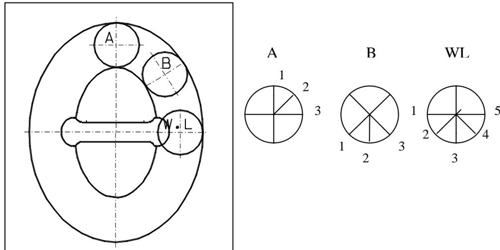
FIGURE 6. Critical regions and respective positions of brittle fracture analysis in studless and stud chain links.
