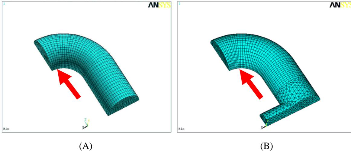
FIGURE 2. Geometries and meshes adopted for the analyses of the studless (A) and stud chain links (B).
