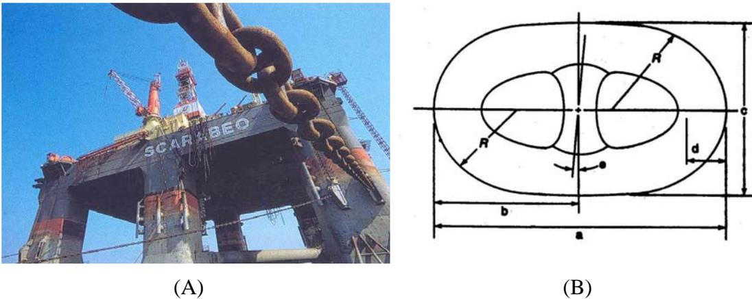
FIGURE 1. Mooring system in an offshore floating structure (A) and an R3 grade stud chain link geometry [1].
