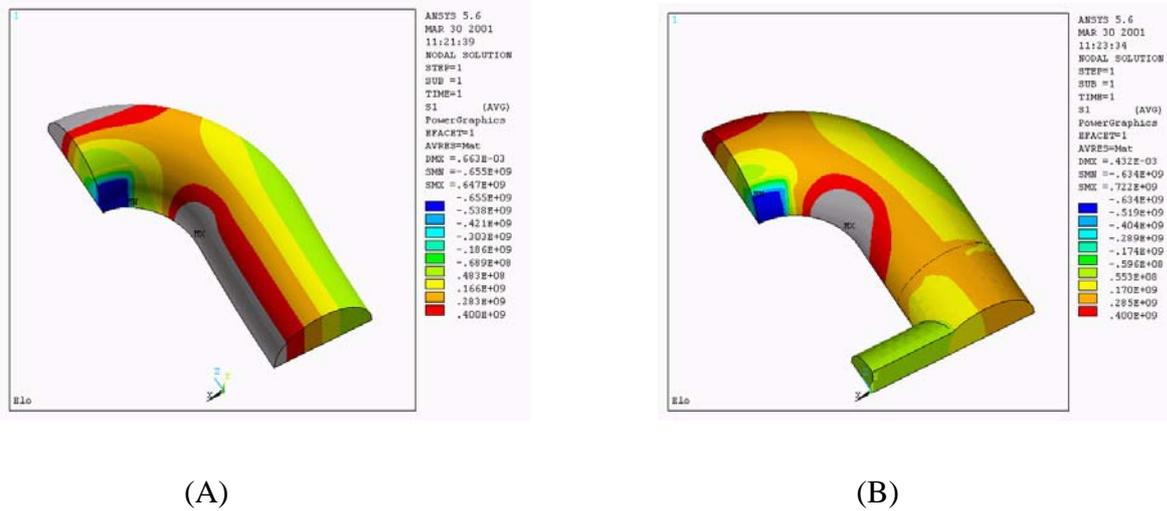
FIGURE 4. Maximum principal stresses smaller than 400 MPa for studless (A) and stud chain links (B).
