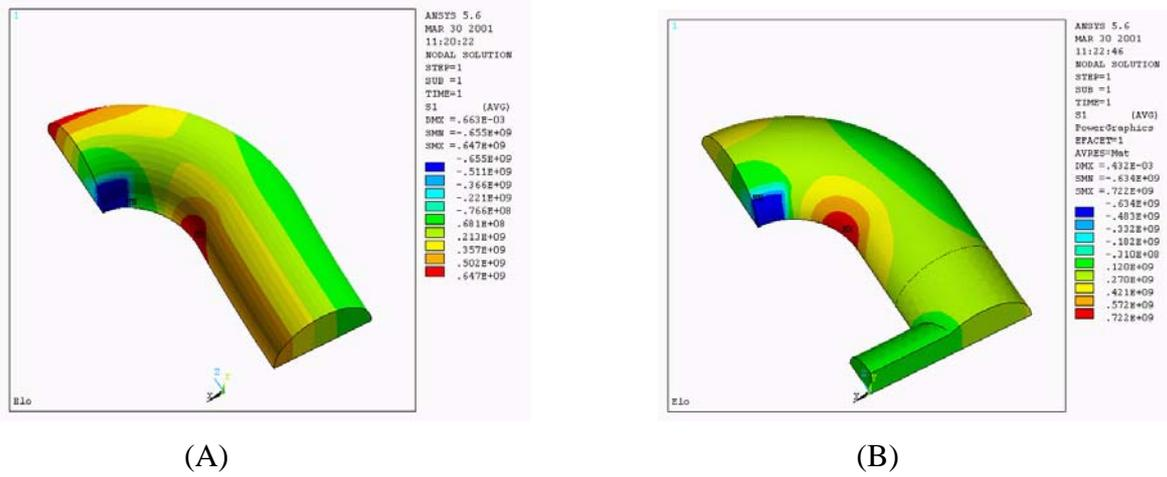
FIGURE 3. Maximum principal stresses for studless (A) and stud chain links (B).
