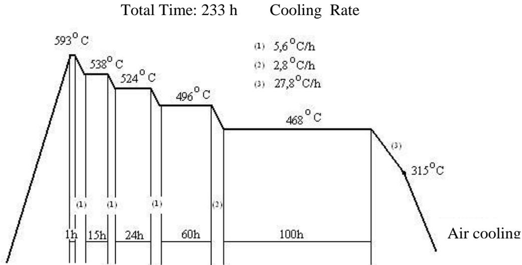
FIGURE 2: Sketch of “Step Cooling” treatment, according to Erwin *et al* [9].
