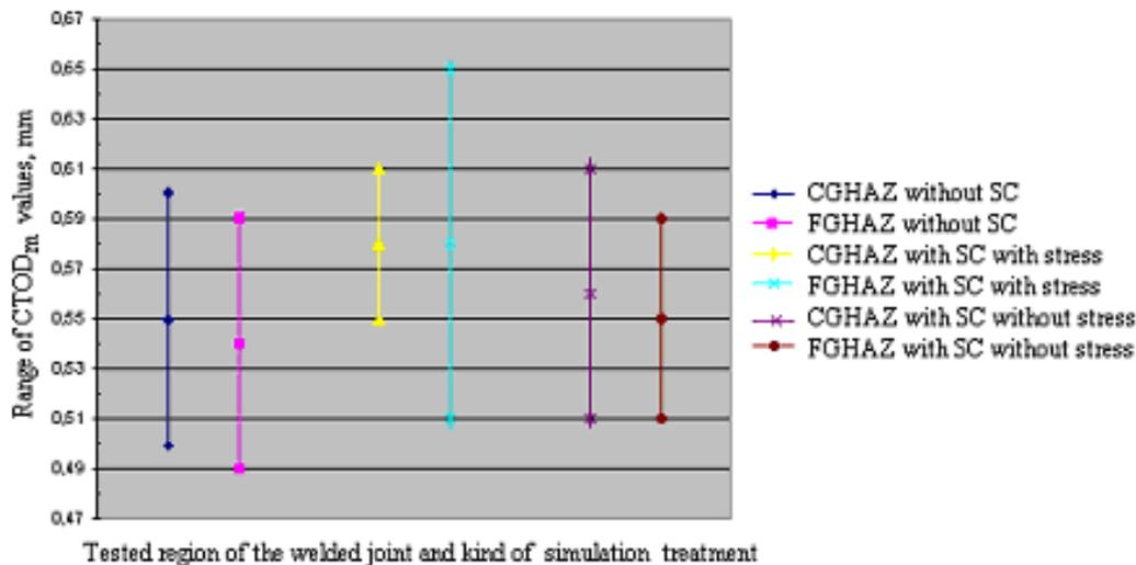
FIGURE 6: Comparison of CTOD<sub>m</sub> values (average  $\pm$  standard deviation) at CGHAZ and at FGHAZ in three treatment conditions (SC = Step Cooling) [11].
