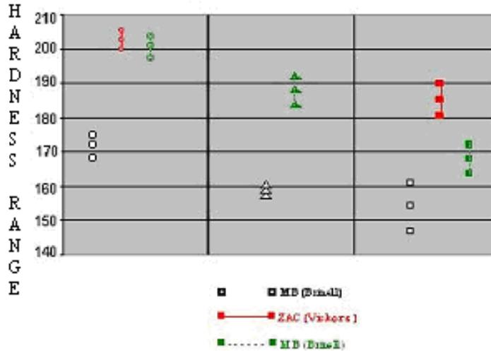
FIGURE 4: Hardness results of different welded joints regions (BM – base metal; HAZ – heat affected zone; WM – weld metal) in each treatment simulation: without Step Cooling (SC), SC without and with stress [11].
