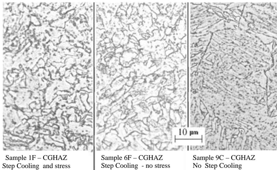
FIGURE 5: Microstructure of CGZAC at three different treatment conditions. Nital 2% - [11].
