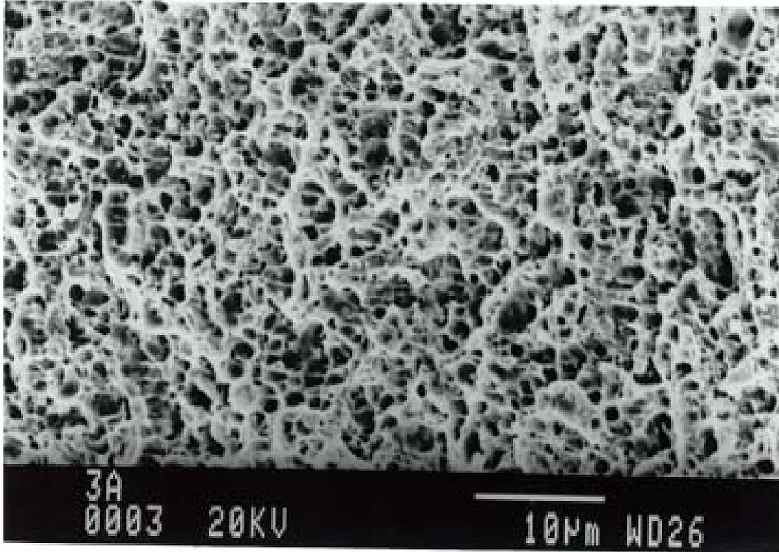
FIGURE 7: Fractography (SEM) of crack surface of CTOD<sub>m</sub> specimens, region of stable crack growth (sample 3A) – FGHAZ – with “Step Cooling” + stress [11].
