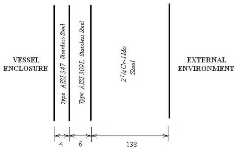
FIGURE 1: Sketch of the HDT wall reactor according to Kessler [1] (dimensions in mm)
