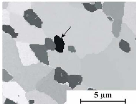
FIGURE.7. EBSD analysis of the grains surrounding the damage site of Fig.6 (b)
