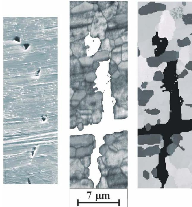
FIGURE.8. SEM micrograph of the damage sites and corresponding EBSD maps
