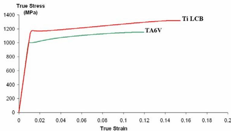
FIGURE 1. True stress - true strain tensile curves of Ti LCB and TA6V
