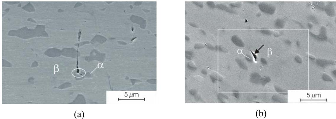
FIGURE.6. Damage sites after  $6.6 \cdot 10^5$  cycles
