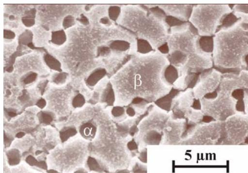
FIGURE 3. Microstructure of the as-received Ti LCB
