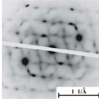
FIGURE. 4 TEM diffraction pattern of the nanometric  $\omega$  phase present within the  $\beta$  phase of the Ti LCB (zone axis  $[012]_{\beta}$ )
