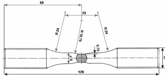
FIGURE 2. Geometry and dimensions of the fatigue samples
