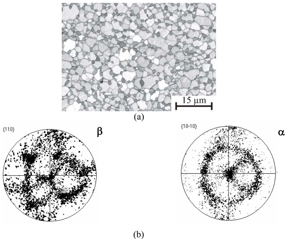
FIGURE.5. (a) : EBSD band contrast map of the Ti LCB ; (b) : EBSD pole figures of the  $\beta$  and  $\alpha$  phases, respectively
