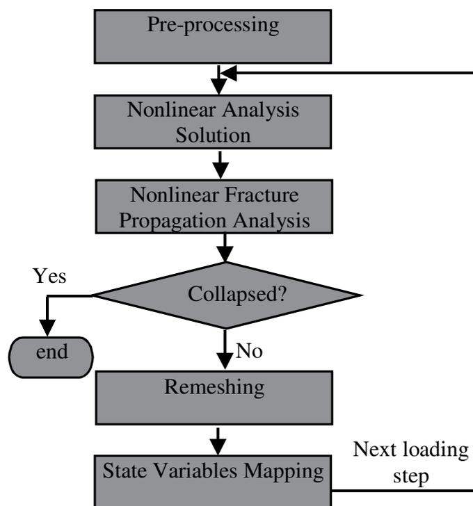
FIGURE.4 Key steps of discrete crack FEM
