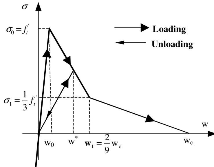
FIGURE. 2 COD- traction curve of nonlinear interface elements
