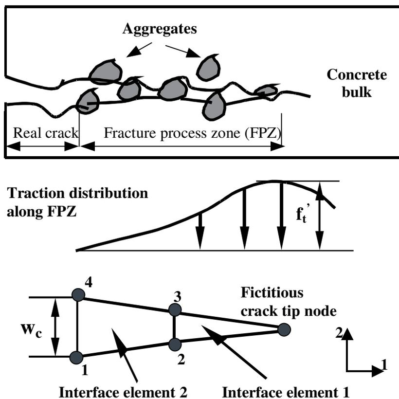
FIGURE. 1 Modelling of FPZ with 4-node interface elements (after Xie [8])
