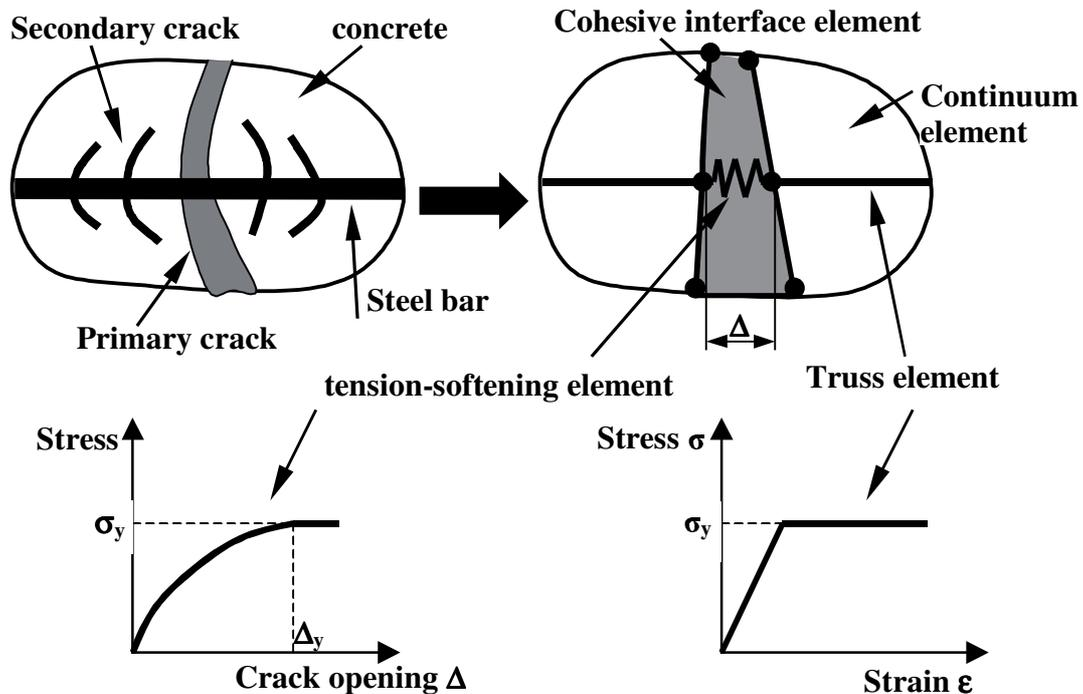
FIGURE. 3 Bond-slip modelling with a tension softening element (after Xie [8])
