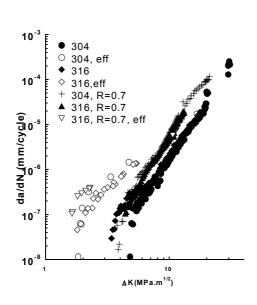
Figure 3: Crack Propagation curves da/dN vs  $\Delta K$  and da/dN vs  $\Delta K_{eff}$  at room temperature for 316L and 304L
