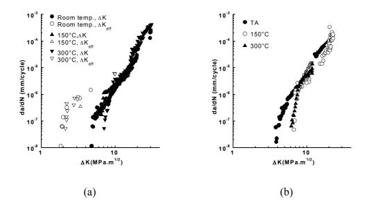
**Figure 5:** Influence of temperature on da/dN vs  $\Delta K$  and da/dN vs  $\Delta K_{eff}$  curves in 304L at R=0.1 (a) and R=0.7 (b).
