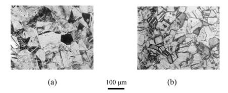
Figure 1: Microstructure of 304L (a) and 316L (b) alloys
