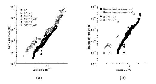
**Figure 6:** Influence of temperature on da/dN vs  $\Delta K$  and da/dN vs  $\Delta K_{eff}$  curves in 316L at R=0.1 (a) and R=0.7 (b).
