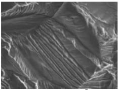
(a)  $150^{\circ}$ C, da/dN = 2  $10^{-7}$  mm/cycle,  $\Delta K = 6.8 \text{ MPa}\sqrt{\text{m}}$
