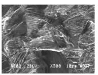
(a) 304L, da/dN =  $6 \ 10^{-8} \text{ mm/cycle}$ ,  $\Delta K = 5.1 \text{ MPa}\sqrt{\text{m}}$ (b) 316L, da/dN =  $1.3 \ 10^{-7} \text{ mm/cycle}$ ,
