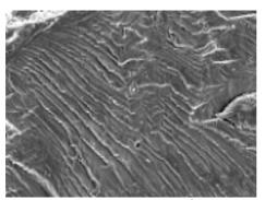
(c)  $150^{\circ}$ C,  $da/dN = 8.10^{-6}$  mm/cycle, (f)  $300^{\circ}$ C,  $da/dN = 1.510^{-6}$  mm/cycle,  $\Delta K = 25 \text{ MPa}\sqrt{\text{m}}$
