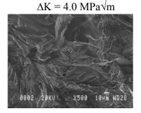
**Figure 4:** Fracture surface morphology in the near-threshold range.
