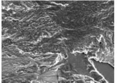
(b)  $150^{\circ}$ C, da/dN = 3.  $10^{-6}$  mm/cycle, (e)  $300^{\circ}$ C, da/dN= $3.10^{-6}$ mm/cycle,  $\Delta K = 12 MPa\sqrt{m}$
