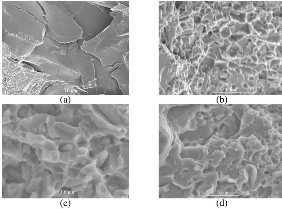
**Figure 4:** Typical fracture surfaces of (a) eutectic carbides, (b) and (c) matrix material subjected to heat treatments 1040-2-s and 1100-2-w resp., and (d) matrix material without secondary carbides
