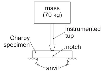
**Figure 2:** Set-up of instrumented drop-weight impact test
