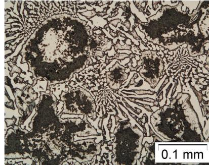
**Figure 1:** Micrograph of the as-cast structure
