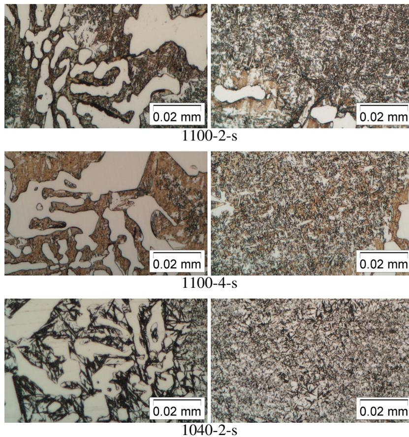
**Figure 3:** Micrographs of the eutectic region (left) and the matrix region (right) after different heat treatments
