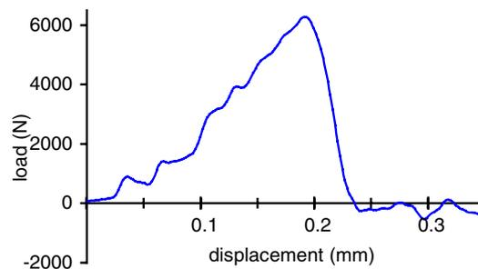
**Figure 5:** Typical load-displacement curve showing overall elastic behaviour of the specimen
